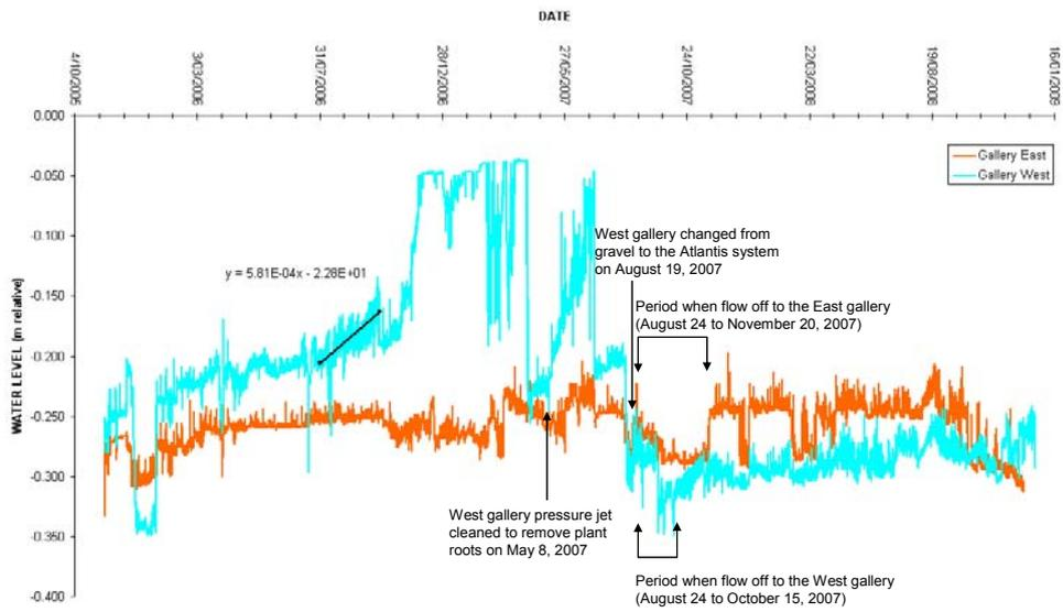
**Figure 7.** Comparison of water levels in the east and west galleries. The periods when inflow of wastewater to the galleries was deliberately off due to the tracer tests in August–October 2007 are labelled on the plot.
