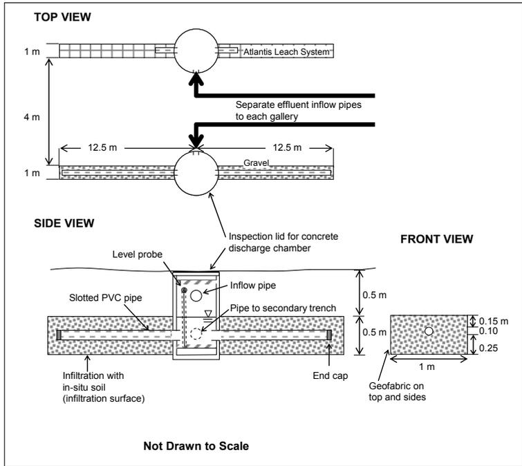
**Figure 2.** Schematic of the covered infiltration galleries as originally installed at the Floreat site
