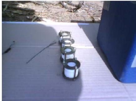
**Figure 5.** Diffusion chambers in field prior to lowering into groundwater for survival experiment
