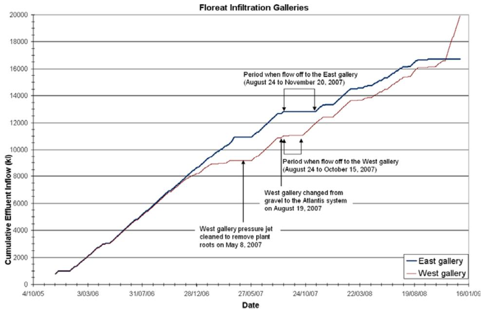
**Figure 6.** The history of cumulative effluent inflow to the infiltration galleries. The west gallery was originally gravel-filled. It was replaced with an Atlantis Leach System<sup>®</sup>, similar to the east gallery, on August 19, 2007.
