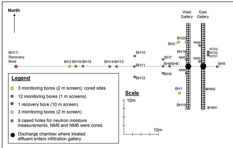
**Figure 4.** Map view of the Floreat site showing the positions of the monitoring bores, the recovery bore, the neutron moisture meter access tubes and the two infiltration galleries
