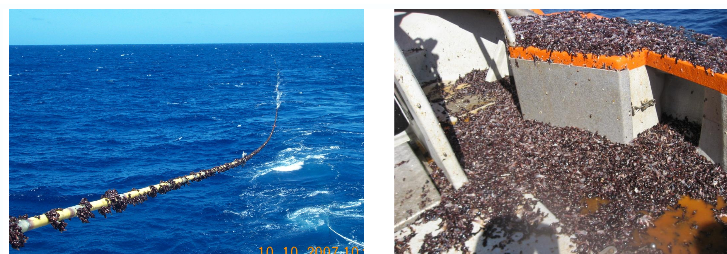
Figure 2. Streamers are fouled by pelagic goose barnacles. Cleaning poses OHSE risks and creates an unpleasant working environment.
