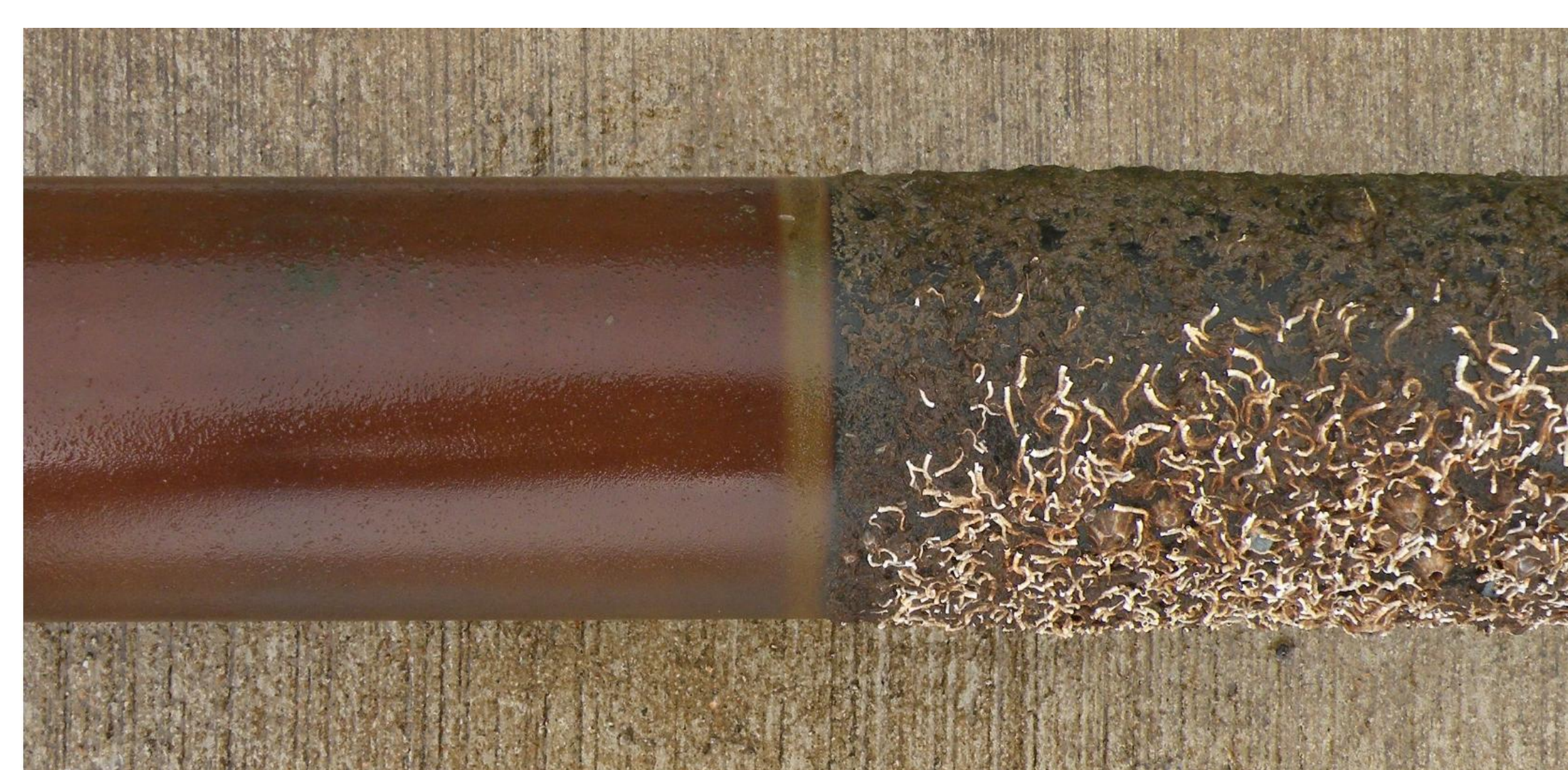
Figure 5. Streamer jacket high-density sample after 210 days field exposure in Townsville Harbour, showing the interface between the sprayed and unsprayed area.
