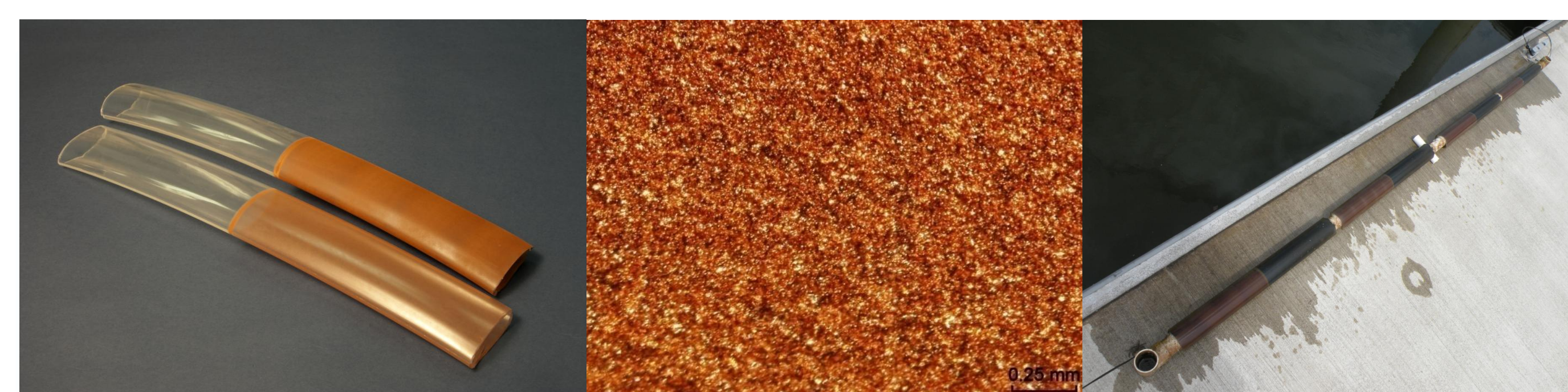
Figure 3, High-density copper coated streamer jacket before deployment, a light micrograph of the surface, and being deployed in Townsville Harbour (L to R).
