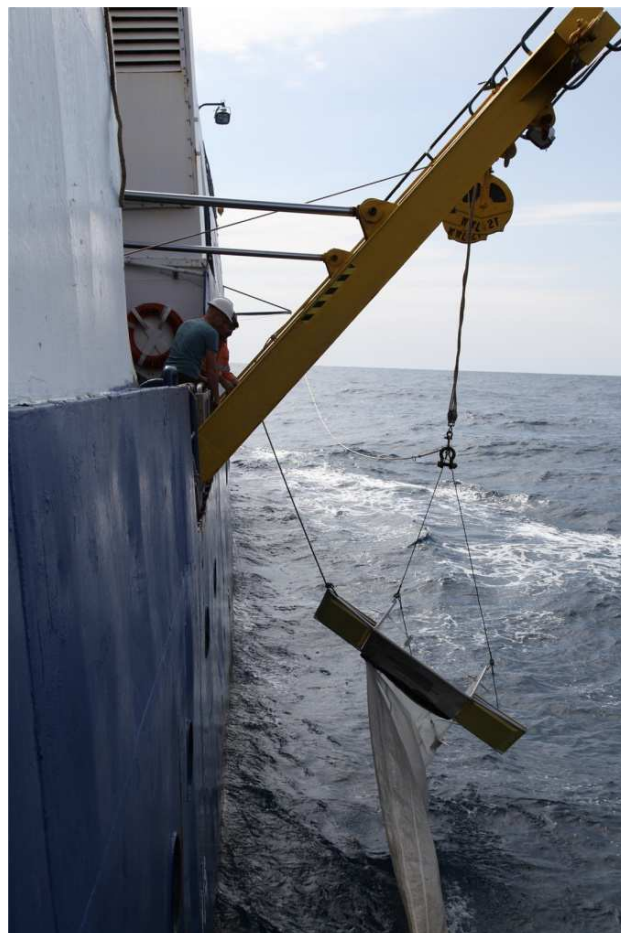
Figure 5. Deploying the surface trawl net aboard the Southern Surveyor
