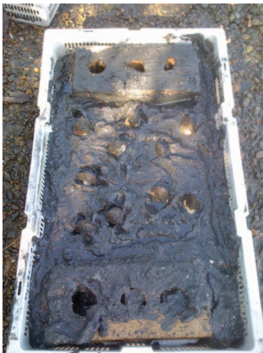
Figure 5.5. Field transplantation cage, about 60 cm × 40 cm × 10 cm.
