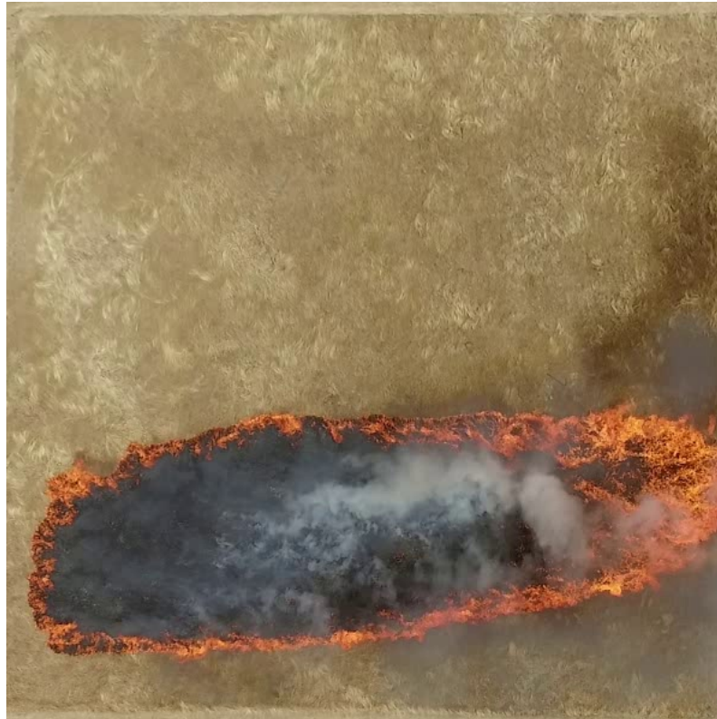
Figure 8. Top- Raw oblique aerial imagery of fire S13 at Braidwood approximately 90 seconds after ignition. Bottom- Spatially rectified and trimmed image used for fire perimeter digitisation and rate of spread measurements.
