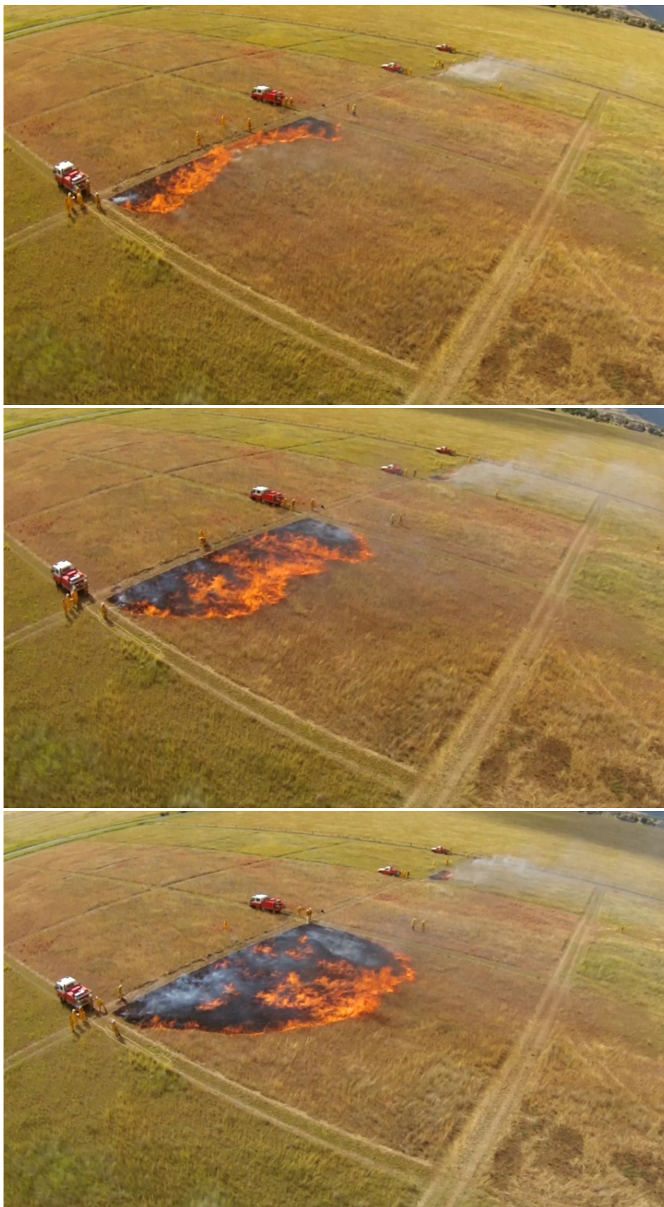
Figure 10. Typical fire behaviour differences observed in a paired burn, Tamworth, NSW. Time since ignition: top image is 20 sec; middle image is 30 sec; bottom image is 40 sec. Images depict plot 5 (background; curing level 48%; sparse fuels) and plot 11 (foreground; 100% cured).
