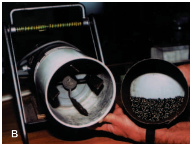
(B) Motor driven scarifier used to pretreat acacia seed
