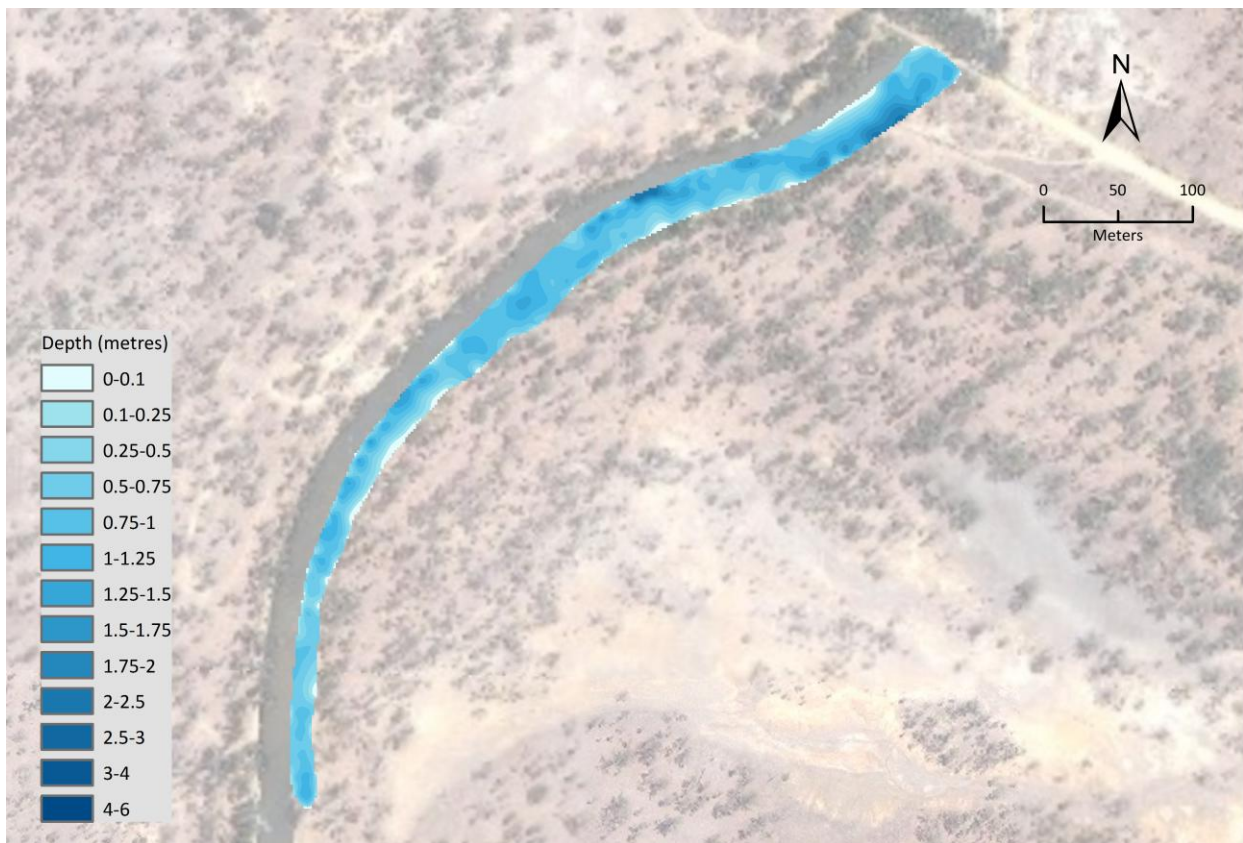
Figure 2 Bathymetry map of waterhole G01. Depth and waterhole perimeter data generated from data collected Oct 2012
