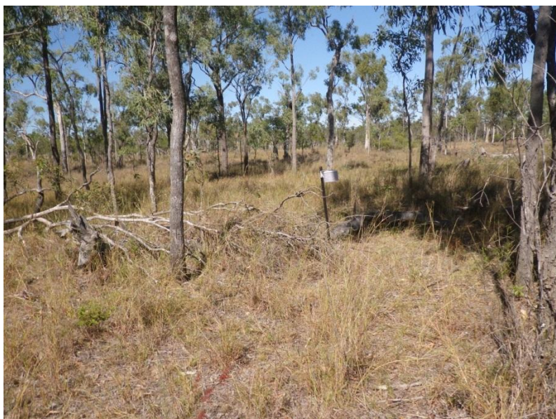
Figure 3.4 Continuous air temperature logger rig with probe fixed to centre of vented solar shield, located in the mid-day shade of several large trees
