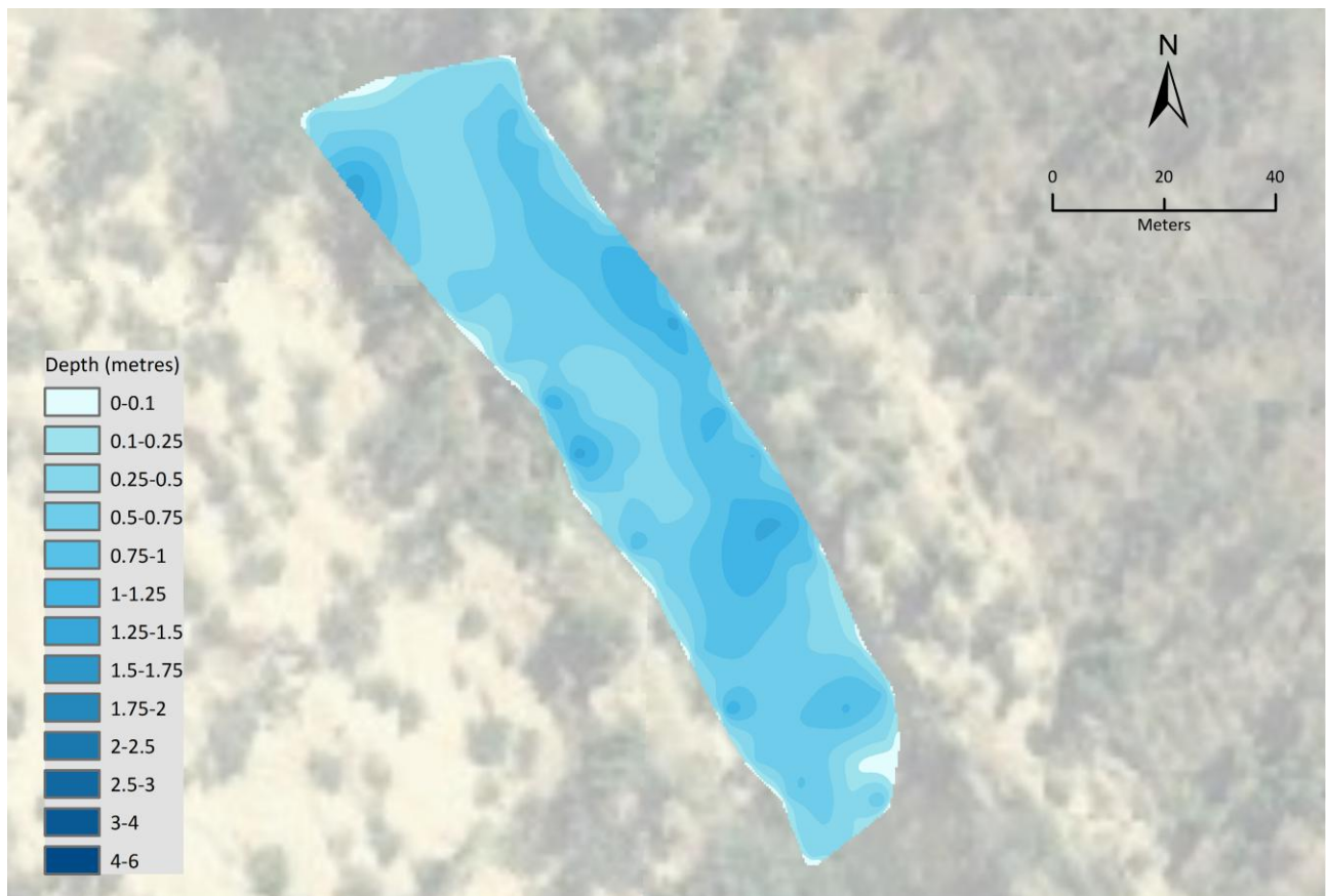
Figure 31 Bathymetry map of waterhole G04. Depth and waterhole perimeter data generated from data collected Oct 2012
