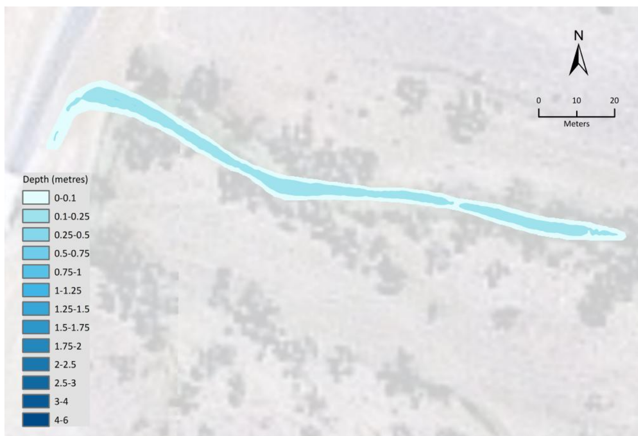
Figure 82 Bathymetry map of waterhole F10. Depth and waterhole perimeter data generated from data collected Oct 2012
