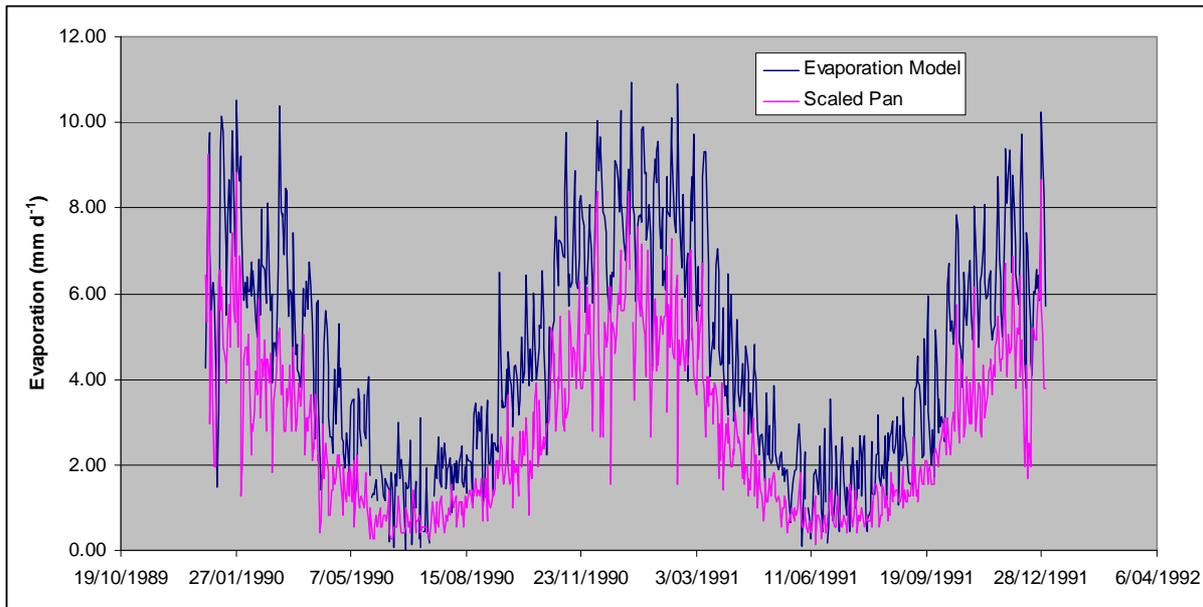
Figure 5-33. Modelled and scaled pan evaporation estimates of evaporation for an irrigation channel in Tatura
