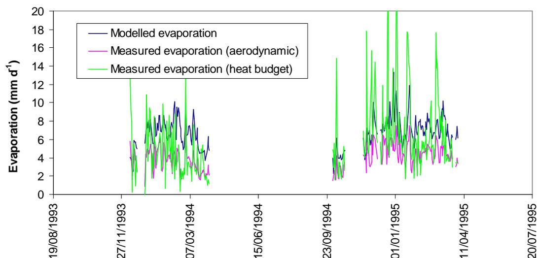
Figure 5-28. Measured and modelled evaporation at Maude Weir (Measured evaporation includes aerodynamic and heat budget approaches.)
