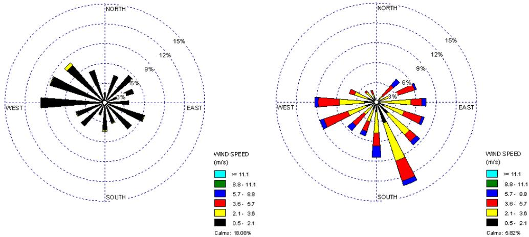
Figure 5-30. Wind roses for wind speed measured over water (left) and over land (right) for January to March 1994
