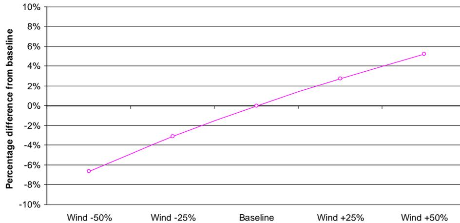
Figure 6-4. Effect of wind speed uncertainty on evaporation estimates
