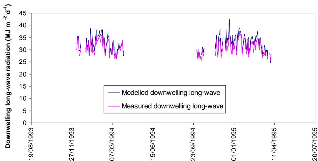
Figure 5-24. Measured and modelled downwelling long-wave radiation at Maude Weir
