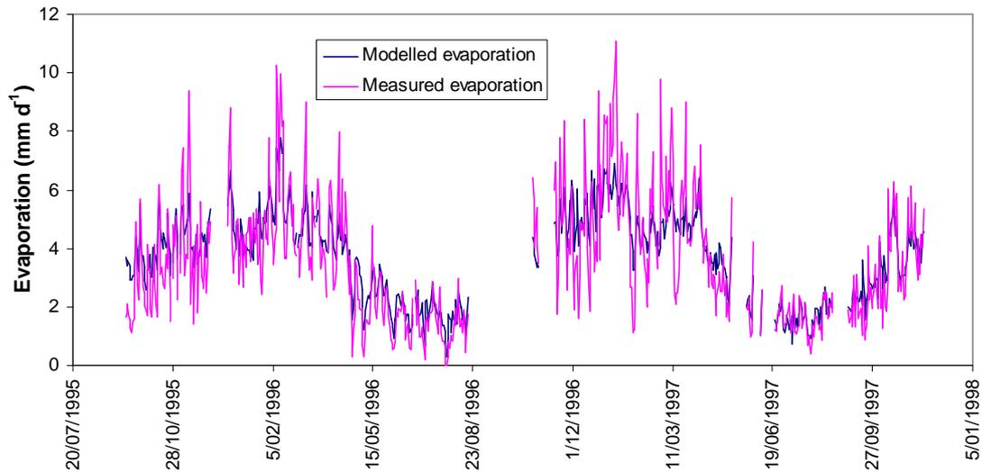
Figure 5-17. Measured and modelled evaporation at Chaffey Dam
