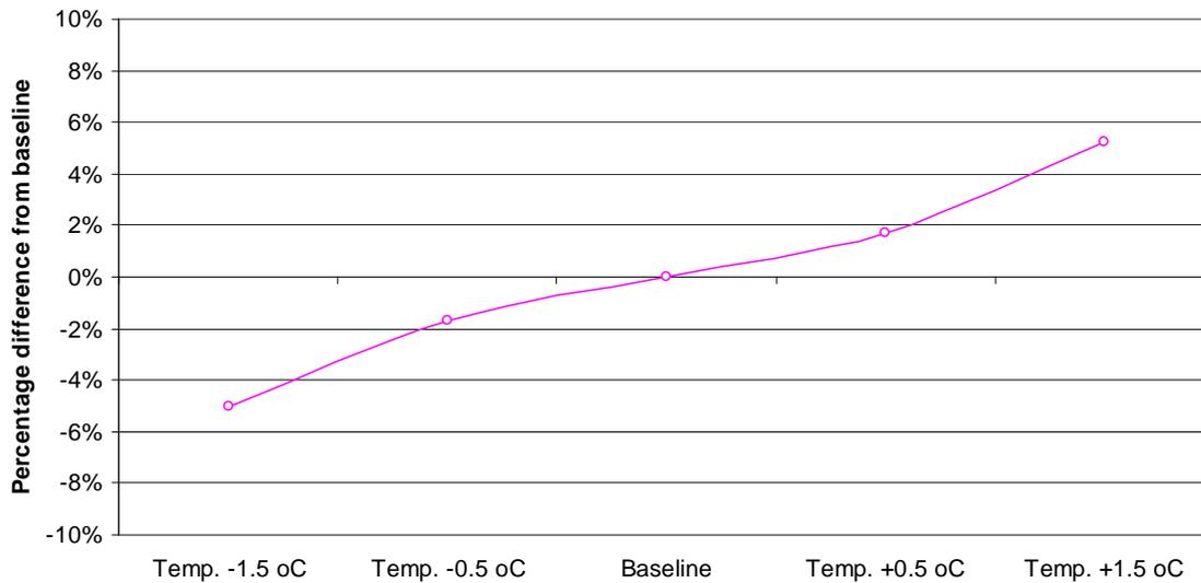
Figure 6-1. Effect of temperature uncertainty on evaporation estimates
