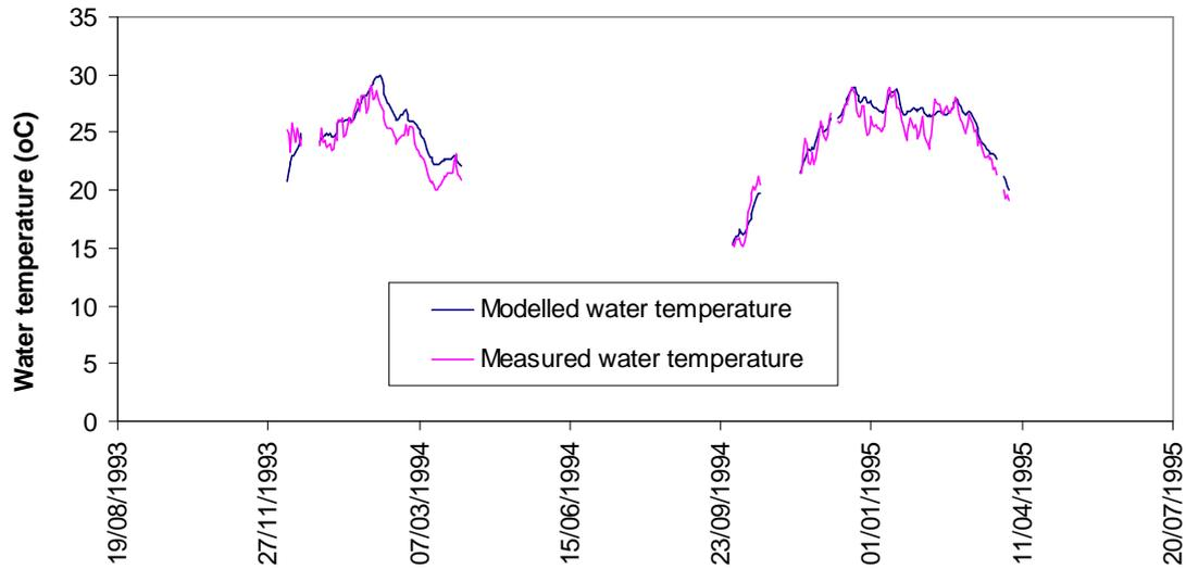
Figure 5-25. Measured and modelled water temperature at Maude Weir
