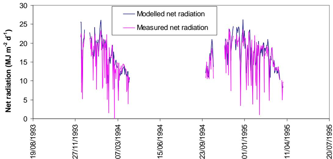
Figure 5-27. Measured and modelled net radiation at Maude Weir
