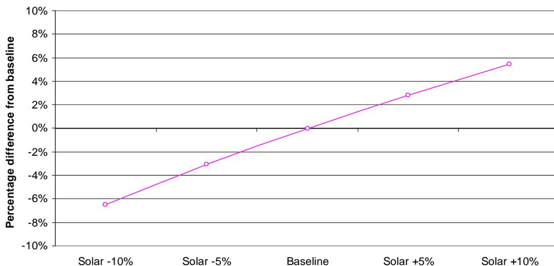
Figure 6-2. Effect of solar radiation uncertainty on evaporation estimates
