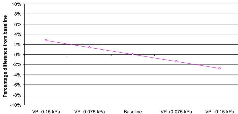
Figure 6-3. Effect of vapour pressure uncertainty on evaporation estimates
