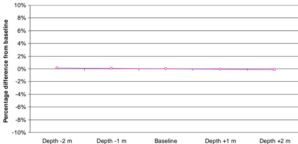
Figure 6-5. Effect of water body depth uncertainty on evaporation estimates
