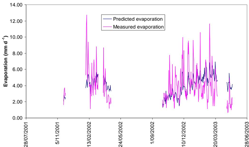
Figure 5-12. Measured and modelled evaporation at Hume Dam
