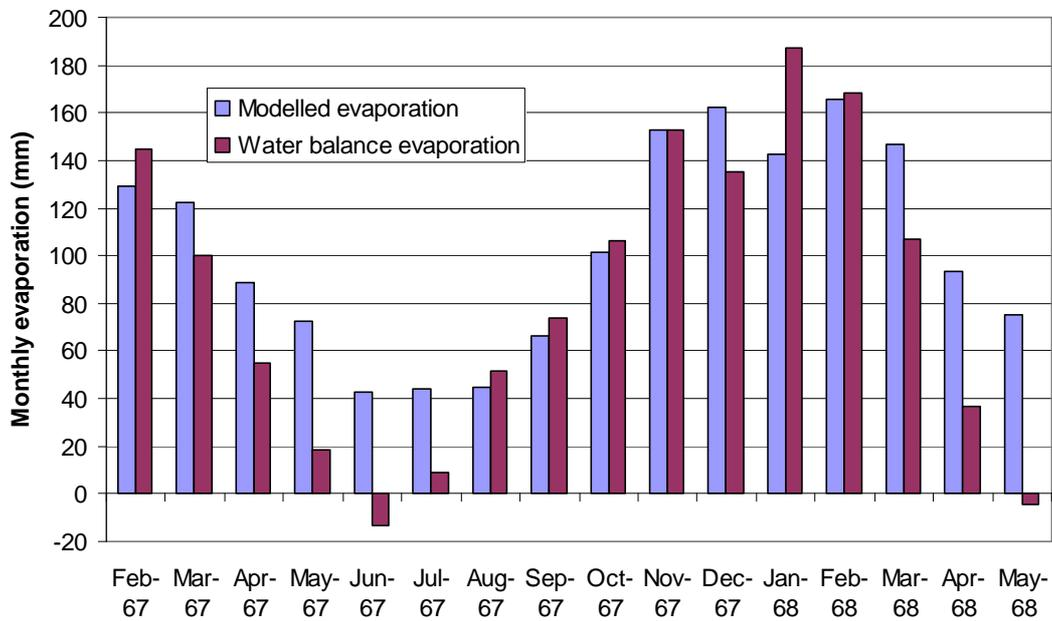
Figure 5-19. Measured and modelled evaporation for Lake Alexandrina and Lake Albert
