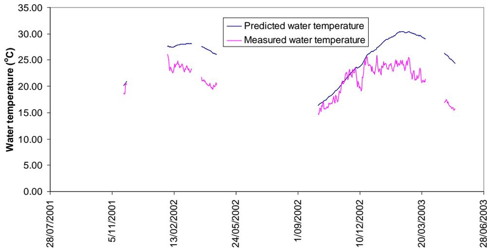
Figure 5-9. Measured and predicted water temperature at Hume Dam
