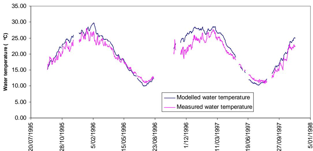
Figure 5-15. Measured and modelled water temperature at Chaffey Dam
