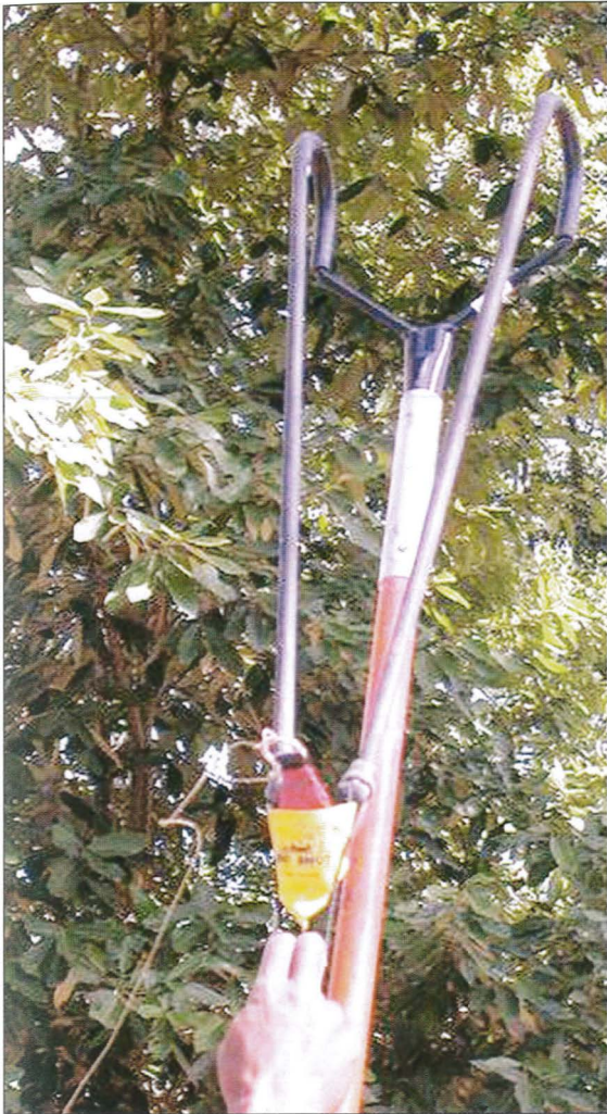
Figure 9. A close-up of the catapult (Big Shot) with a red projectile, attached to a fishing line, placed in yellow sling.
