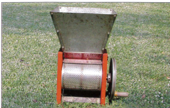
Figure 15. A coffee depulper can be used to remove the pulp of fruit of a size similar to coffee beans.
