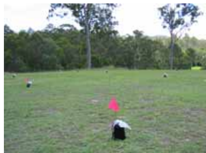
Our first large-scale outdoor deployment in early 2003, joint work with Dartmouth College. Using Mica nodes in Ziploc bags sitting on upturned plastic flower pots in order to raise the antennas above the ground
