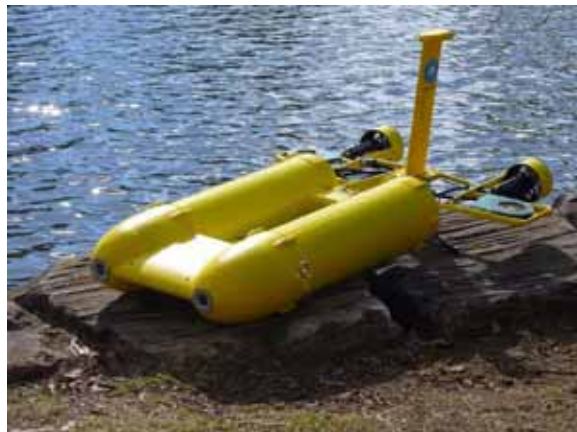
Starbug Mk 2 with integrated Fleck™ for sensor network interaction
