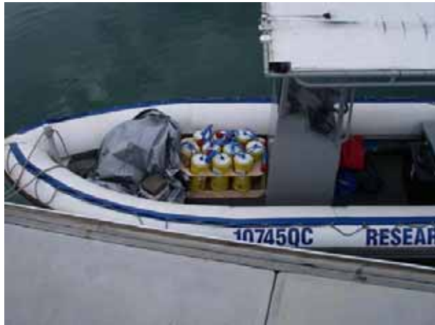
10 acoustic nodes ready for deployment in Moreton Bay for ad-hoc networking trials
