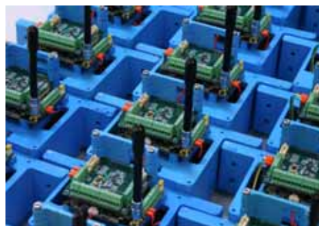
Current generation wireless sensor nodes during assembly, Fleck3™ base boards with moisture sensor interface boards
