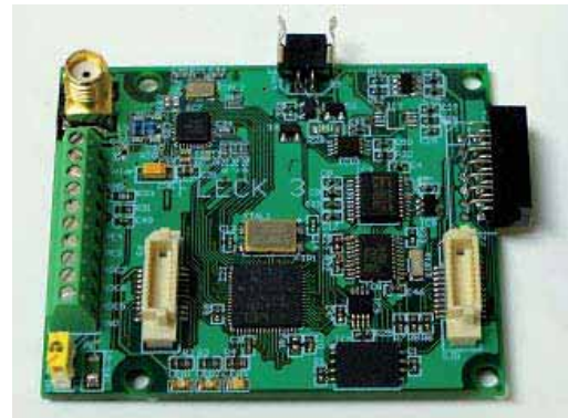
Fleck™ 3B sensor network node.
