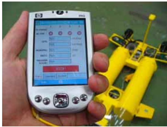
PDA providing wireless communications and network interface to robots
