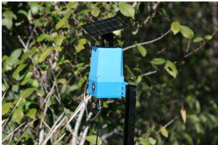
Current generation CSIRO node in environmental housing with solar cell on top
