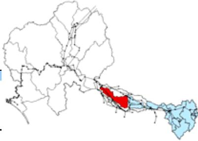
Accounts cannot be established for this reach. The gauged outflows are much greater (by an order of magnitude) than the inflows. The inflows, however, match the outflows of the reach above. It appears that the outflow gauge may be faulty.
