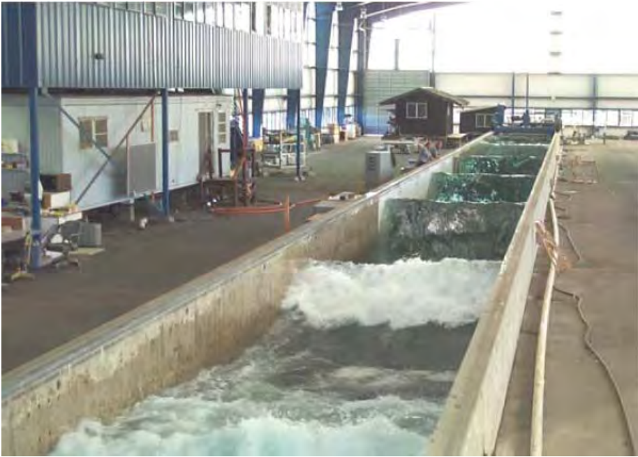
Figure 8-15 Oregon State University Wave Research Lab used to develop the Linear Direct-Drive Wave Energy Generator [202].
