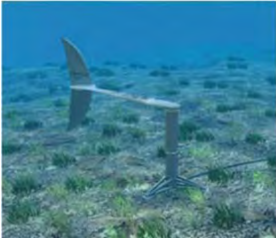
Figure 4-34 BioPower bioStream oscillating hydrofoil. Copyright BioPower [57].
