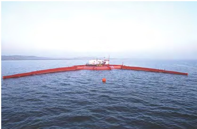
Figure 4-13 Wave Dragon prototype showing tapered channel and ramp. Image courtesy of Wave Dragon [34].
