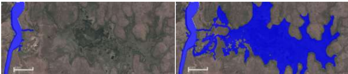
Figure 6 Bathtub fills of the South Alligator River and Boggy Plain for elevations of 3.2 m (left) and 3.3 m (right) AHD.
