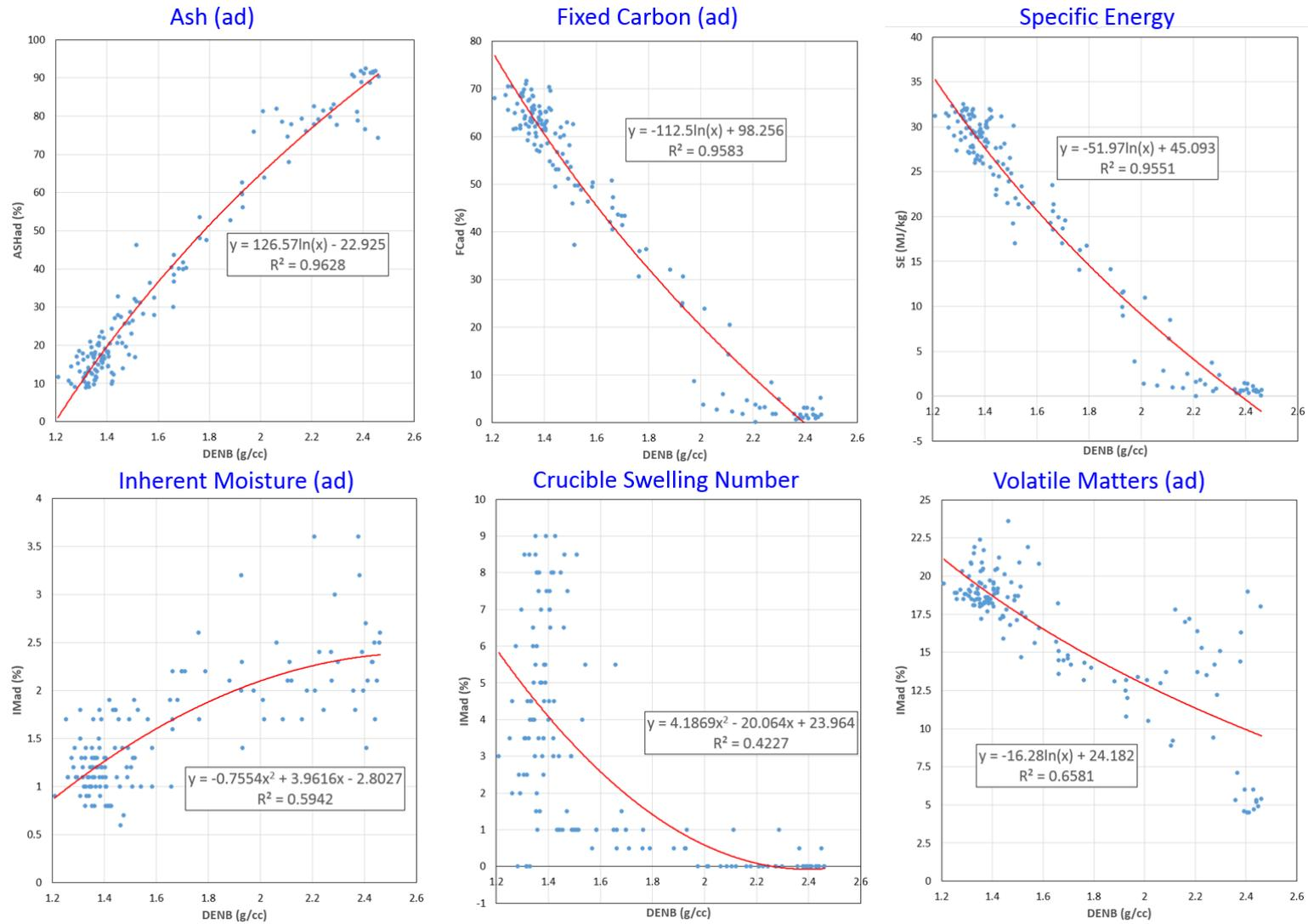
Figure 10 Correlations of laboratory coal quality parameters with the geophysical density log DENB: ash, fixed carbon, specific energy, inherent moisture, crucible number and volatile matters.
