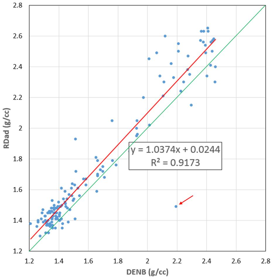
Figure 7 The crossplot of the laboratory measured relative density (RDad) and the geophysical density log (DENB). The red line is the fitted curve while the green line shows the expected fitting curve.
