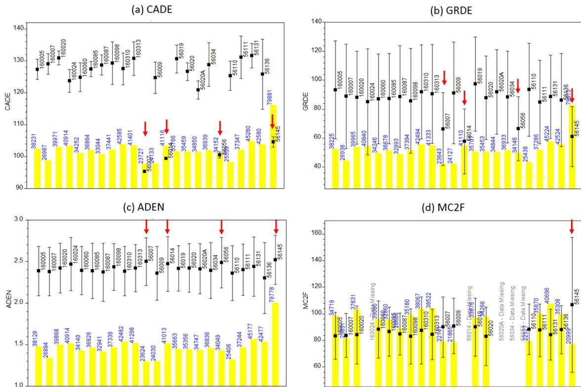
Figure 20 Averages and standard deviations of geophysical logs from BMA: (a) calliper CADE, (b) natural gamma GRDE, (c) short spaced density ADEN, and (d) sonic MC2F from different boreholes. The yellow bars with blue numbers indicate the sample counts for the statistical computations.
