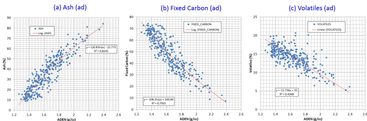
**Figure 26 Cross-correlations of coal quality parameters with the geophysical log ADEN: (a) Ash content; (b) Fixed carbon; (c) Volatile matters.**
