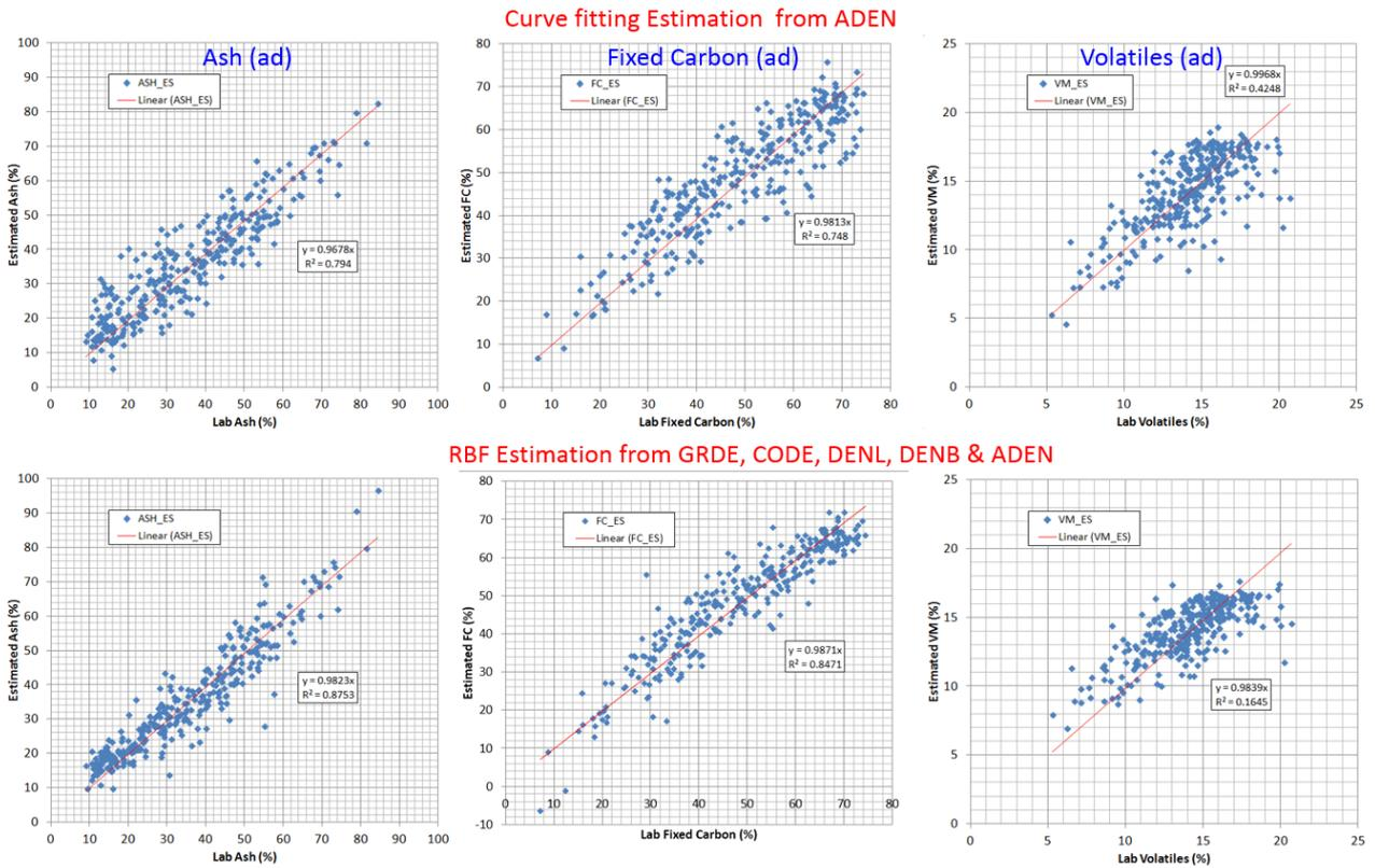
Figure 27 The estimated air-dry ash, fixed carbon and volatile matters from a single geophysical log ADEN (top row) and multiple geophysical logs (bottom row).
