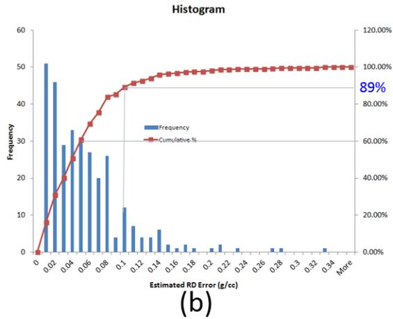
Figure 25 The error histograms for the estimated RDs from (a) the single density log ADEN; and (b) multiple geophysical logs. It is clear that the estimation errors from multiple geophysical logs are more concentrated in the lower end than those from the single density log.
