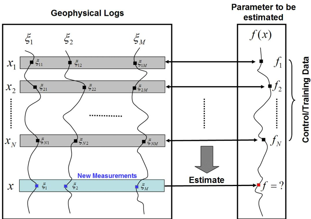
Figure 2 Illustration of parameter estimation using multiple geophysical logs. The discrete control data are used to train the parameter estimation algorithm and the trained algorithm is then used to estimate the target parameters with new measurements.
