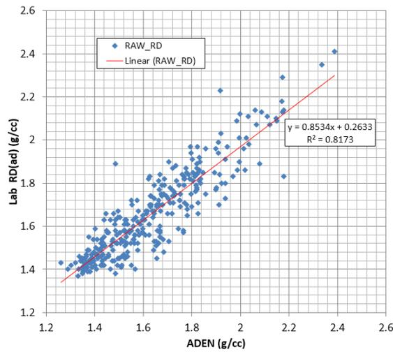
Figure 23 The cross-plot of the laboratory RD with the geophysical log ADEN.
