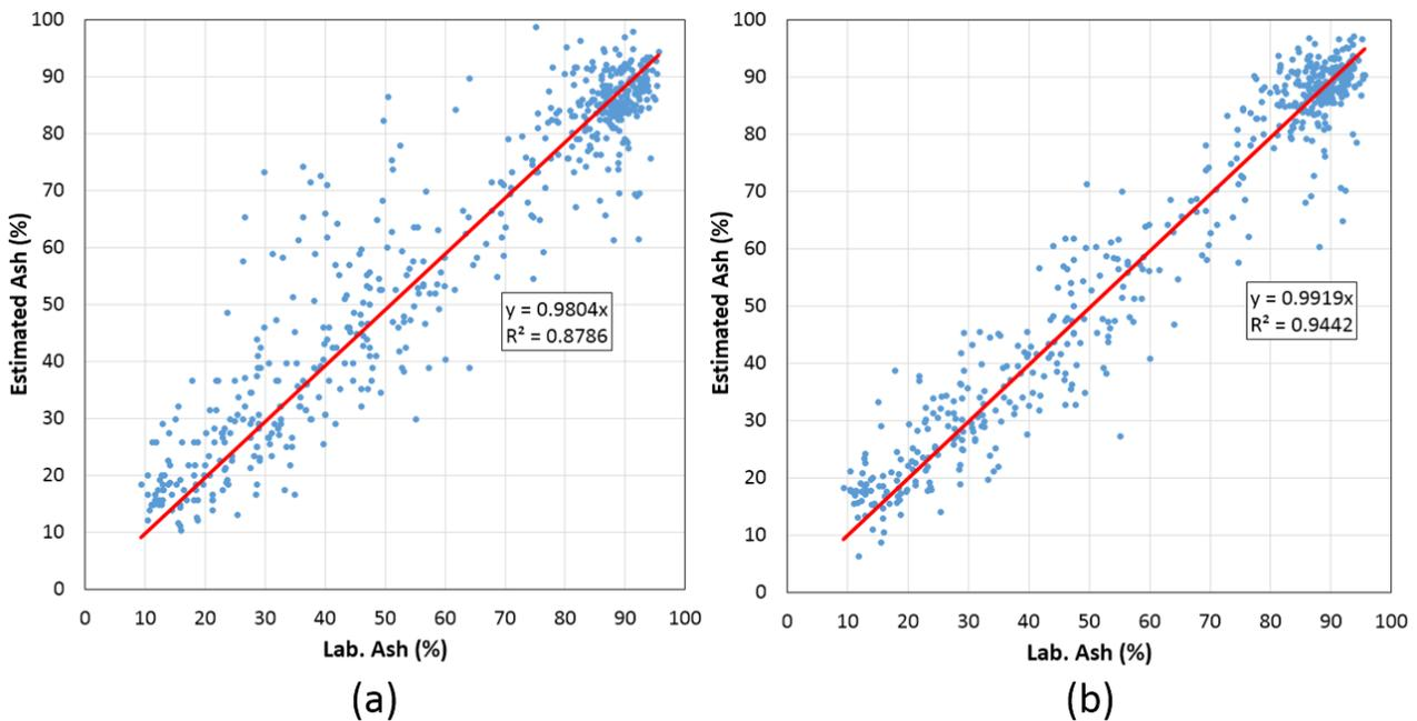
**Figure 29 Cross-correlations of the laboratory measured ashes with the ashes estimated from: (a) the single geophysical density log ADEN; (b) the multi-geophysical logs of GRDE, DENB, DENL, CODE, ADEN, DEPO, MC2F, MC4F, FE1 and FE2.**
