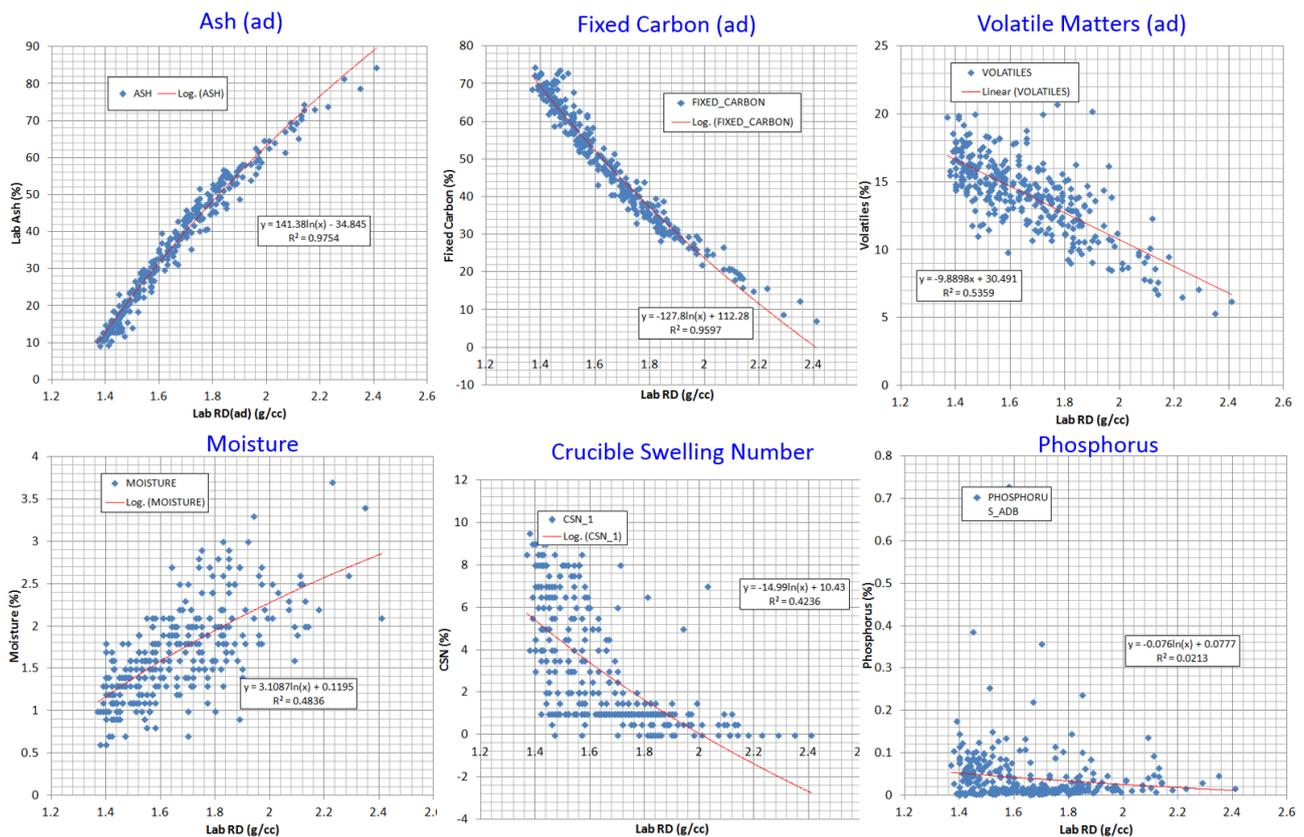
Figure 19 Correlations of laboratory coal quality parameters with relative density (after data samples with wild ash values are excluded). The regressions are in trends observed normally, suggesting the measured ash coal quality parameters and relative densities are in good quality. There are some degrees of scattering.
