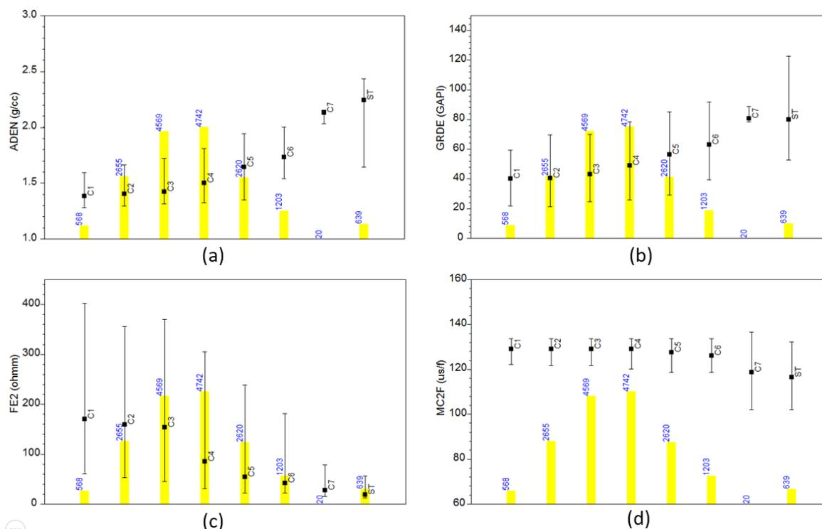
Figure 32 The medians and spreads of the geophysical logs for different lithotypes from the control boreholes in Area 1: (a) Density log ADEN; (b) Gamma ray GRDE; (c) Resistivity log FE2; and (d) Sonic log MC2F. The yellow bars indicate the number of samples used for computation of the statistics for each lithotype and log.
