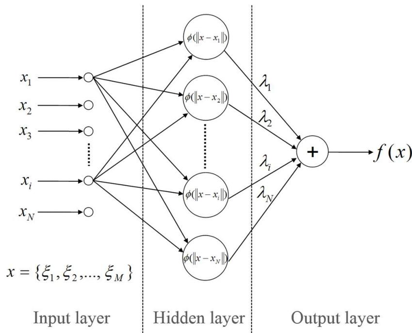
**Figure 3 Schematic illustration of the RBF algorithm expressed by equations (1) and (2). It can be considered as a single layer neural network.**
