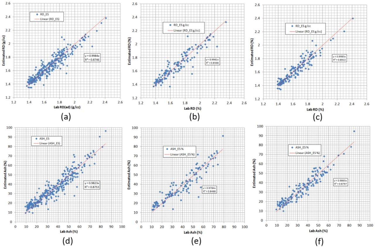
Figure 30 Estimated coal parameters from geophysical logs GRDE, CODE, DENL, DEPO & ADEN for different data sets: (a) Estimated RDs for whole data set; (b) Estimated RDs for Sub-set 1; (c) Estimated RDs for Sub-set 2 using Sub-set 1 as control data; (d) Estimated ash contents for whole data set; (e) Estimated ash contents for Sub-set 1; (f) Estimated ash contents for Sub-set 2 using Sub-set 1 as control data.
