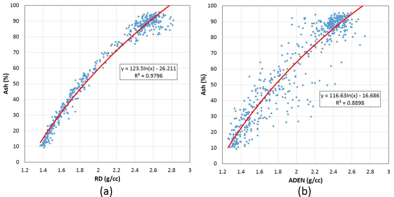
Figure 28 The cross-correlations of laboratory air-dried ashes with (a) the laboratory air-dried relative density RD and (b) the geophysical density log ADEN. Data samples with wild ash values are excluded from the data set. The cross-plot in (b) is more scattered than the one in (a), suggesting that the density log ADEN is more variable than the laboratory measured relative density RD.
