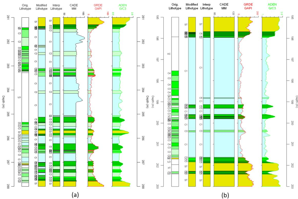
Figure 36 The LogTrans classification of the modified lithotypes using density log ADEN, gamma ray GRDE, resistivity log FE2 and sonic log MC2F for the control holes in Area 1: (a) 16005 & (b) 160098. Shown from the left to the right: original lithotypes provided by the mine; modified lithotypes; interpreted lithotypes using LogTrans based on the training statistics in Figure 32; followed by logs calliper CADE, gamma ray GRDE and density log ADEN.
