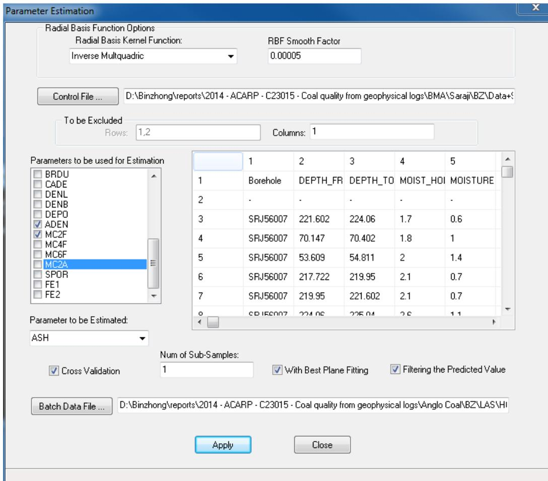
Figure 4 User interface of new RBF-based algorithm developed for coal quality parameter estimation from geophysical logs.
