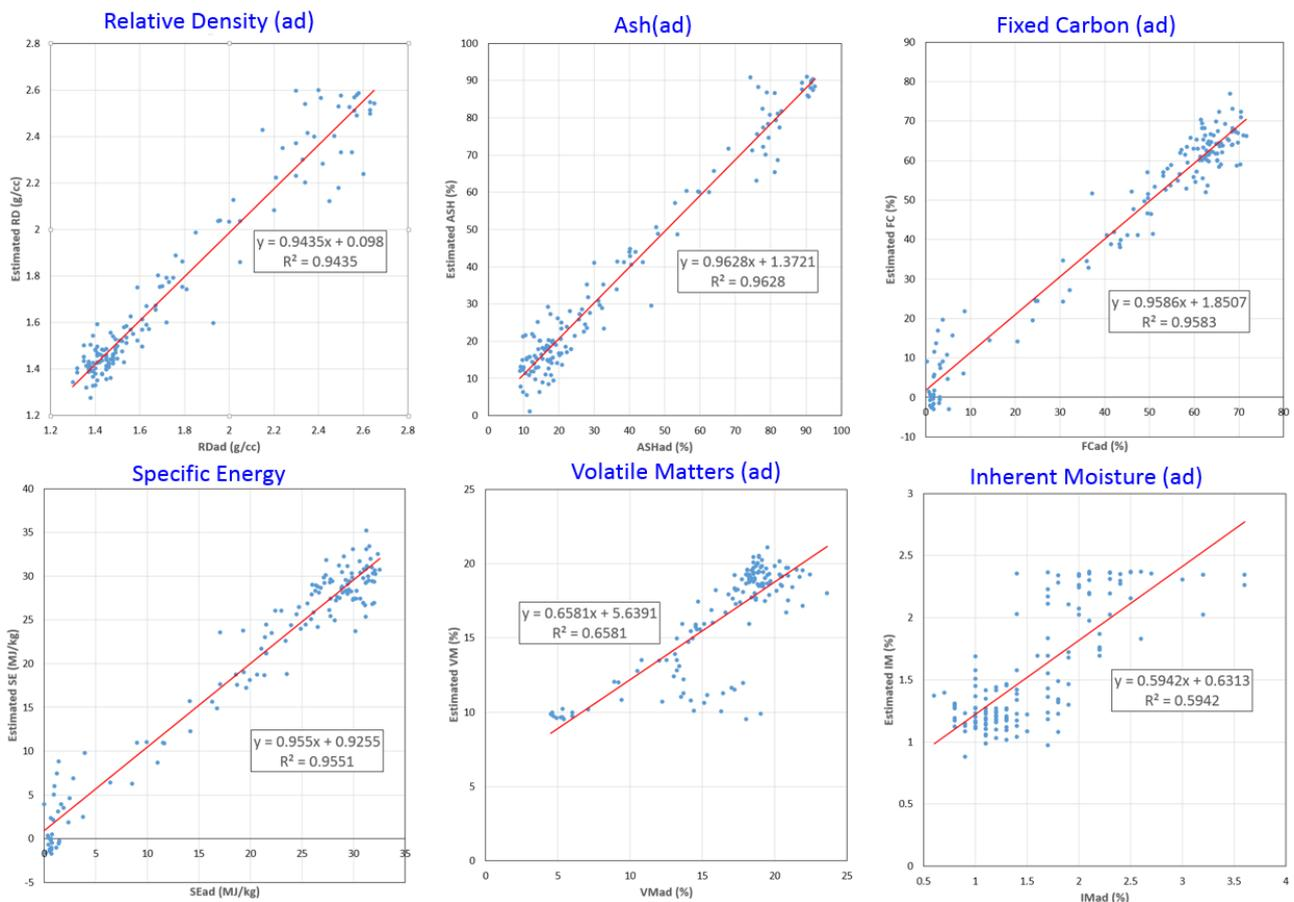
Figure 14 The cross-plots of the laboratory coal quality parameters with the corresponding coal quality parameters estimated from geophysical density log DENB.
