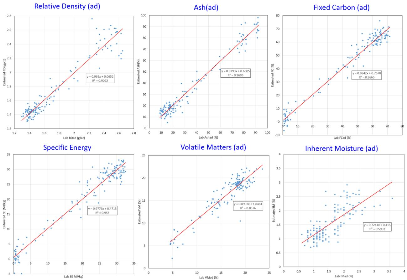
Figure 15 The cross-plots of the laboratory coal quality parameters with the corresponding coal quality parameters estimated from multi geophysical logs: GRDE DENL, DENB, DEPO, MC2F, MC4F, GRNP & RPOR.
