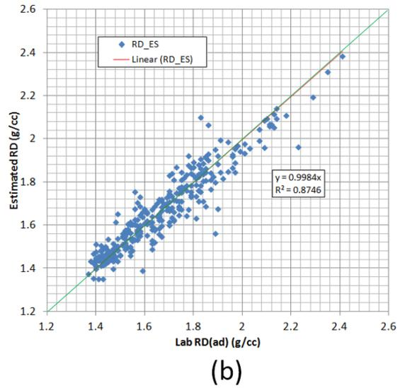
Figure 24 The cross plot of the estimated density RD with the laboratory RD: (a) Estimated from a single density log ADEN; (b) Estimated from multiple geophysical logs GRDE, CODE, DENL and ADEN. The red line is the linear-fitted curve while the green line shows the expected fitting curve.
