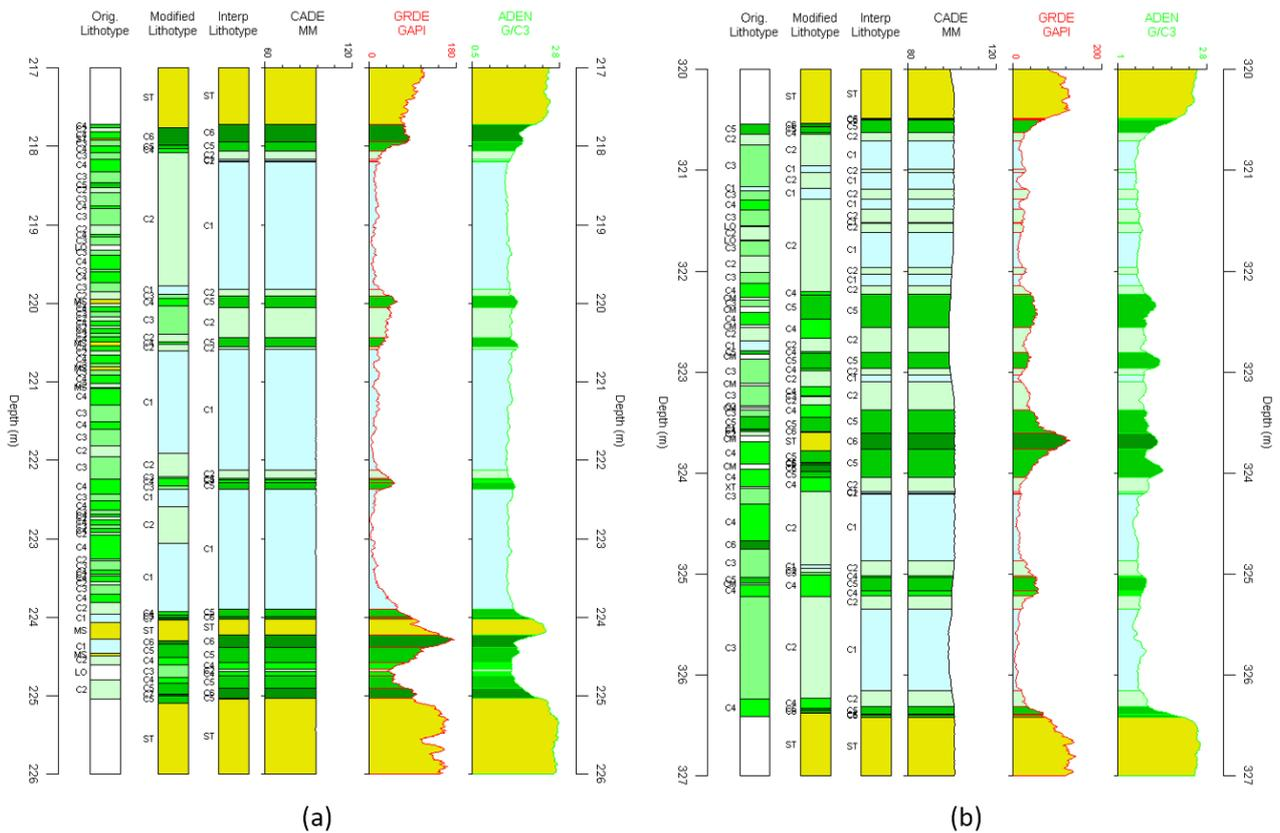
**Figure 37** The LogTrans classification of the modified lithotypes using density log ADEN, gamma ray GRDE, resistivity log FE2 and sonic log MC2F for independent holes in Area 2: (a) 56007 & (b) 56056. Shown from the left to the right: original lithotypes provided by the mine; modified lithotypes; interpreted lithotypes using LogTrans based on the training statistics in Figure 32; followed by logs calliper CADE, gamma ray GRDE and density log ADEN.
