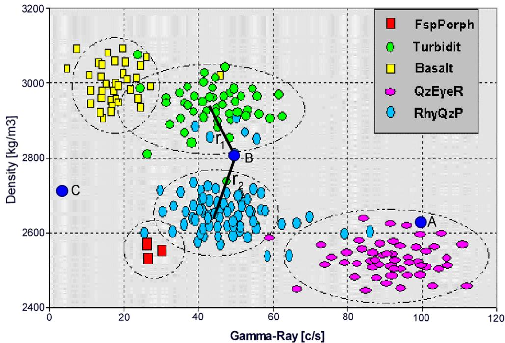
Figure B - 1 Hypothetical control data set, to illustrate the LogTrans algorithm (modified after Emilsson, 1993). Points A, B, C define (density, gamma) data pairs recorded in non-control holes. LogTrans interprets A, B, C as belonging to the nearest rock class domain on the control data scatterplot.
