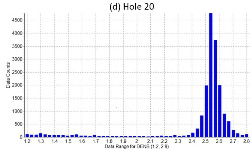
Figure 13 The histograms of geophysical density log DENB for boreholes: (a) Hole 01; (b) Hole 05; (c) Hole 12; (d) Hole 20.
