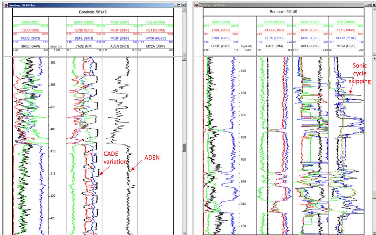
Figure 22 The geophysical logs from Borehole 56145. Left: The borehole diameter (CADE) variation has no significant effect on density log ADEN; Right: There are evident cycle skipping events with sonic logs MC2F, MC4F, MC6F and MC2A.
