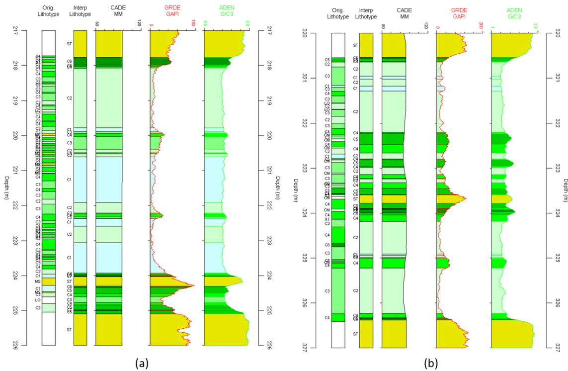
Figure 34 The LogTrans lithotype classification using density log ADEN, gamma ray GRDE, resistivity log FE2 and sonic log MC2F for independent holes in Area 2: (a) 56007 & (b) 56056. Shown from the left to the right: original lithotypes provided by the mine; interpreted lithotypes using LogTrans based on the training statistics in Figure 32; followed by logs caller CADE, gamma ray GRDE and density log ADEN.
