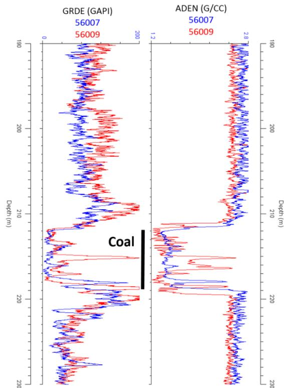
Figure 21 Comparison of the geophysical logs from borehole 56007 (blue) and 56009 (red). The log values of GRDE and ADEN from these two boreholes are very close at the coal seam level in spite of the slightly different values for surrounding rocks.
