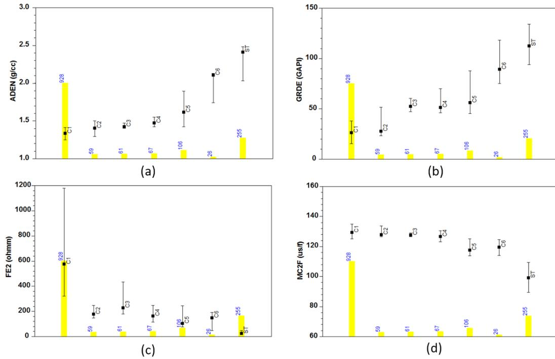
Figure 35 The medians and spreads of the geophysical logs for the modified lithotypes from the control boreholes 16005 & 160098 in Area 1: (a) Density log ADEN; (b) Gamma ray GRDE; (c) Resistivity log FE2; and (d) Sonic log MC2F. The yellow bars indicate the number of samples used for computation of the statistics for each lithotype and log.
