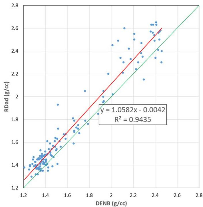
Figure 9 The correlation of the laboratory measured relative density RD and the geophysical density log DENB. The red line is the fitted curve while the green line shows the expected fitting curve.
