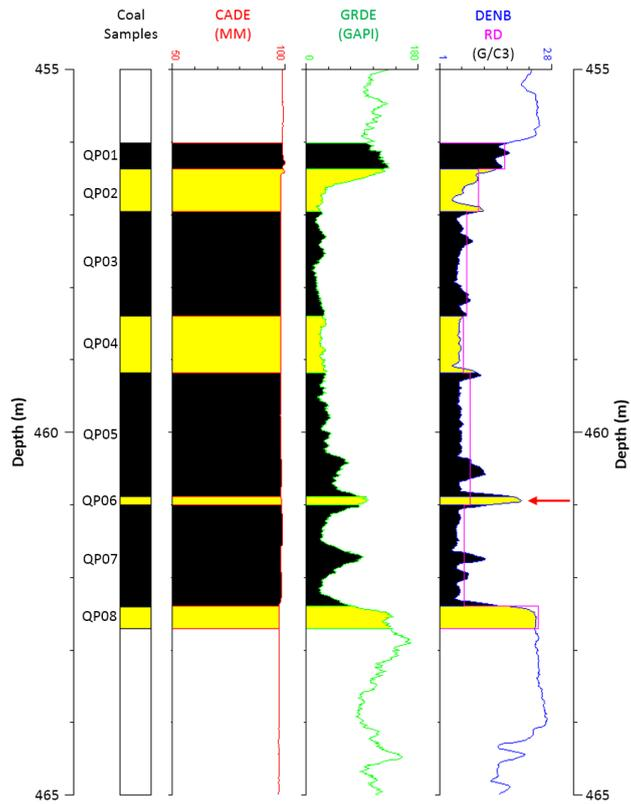
Figure 8 Coal samples and geophysical logs for borehole Hole10 from Anglo American. The magenta curve on the 4<sup>th</sup> column shows the relative density (RD) measured in laboratory. The RD of sample QP06 is much smaller than the geophysical density log value for the sample.
