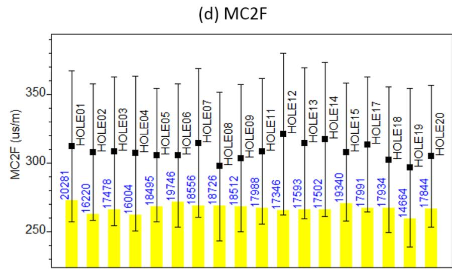
Figure 11 Averages and standard deviations of geophysical logs from Anglo American: (a) calliper CADE, (b) natural gamma GRDE, (c) short spaced density DENB, and (d) sonic MC2F from different boreholes. The yellow bars with blue numbers indicate the sample counts for the statistical computations.
