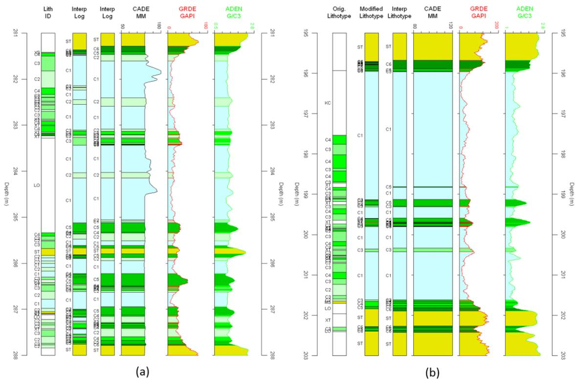
Figure 33 The LogTrans lithotype classification using density log ADEN, gamma ray GRDE, resistivity log FE2 and sonic log MC2F for the control holes in Area 1: (a) 16005 & (b) 160098. Shown from the left to the right: original lithotypes provided by the mine; interpreted lithotypes using LogTrans based on the training statistics in Figure 32; followed by logs caller CADE, gamma ray GRDE and density log ADEN.
