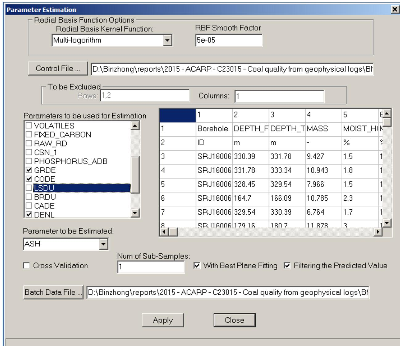
Figure A - 1 User interface of new RBF-based algorithm developed for coal quality parameter estimation from geophysical logs.
