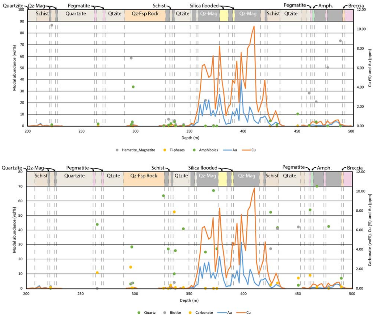
Figure 6: (a) Hematite/magnetite, total Ti phase, and amphibole abundance from TIMA data, and Au and Cu concentration from assay data plotted for drill hole TTNQ364; (b) as for a, but quartz, biotite, and total carbonate abundance.
