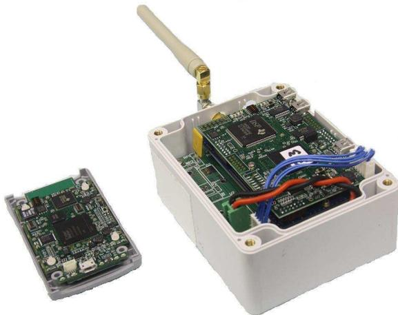
Fig. 3. Two versions of the WASP node.
