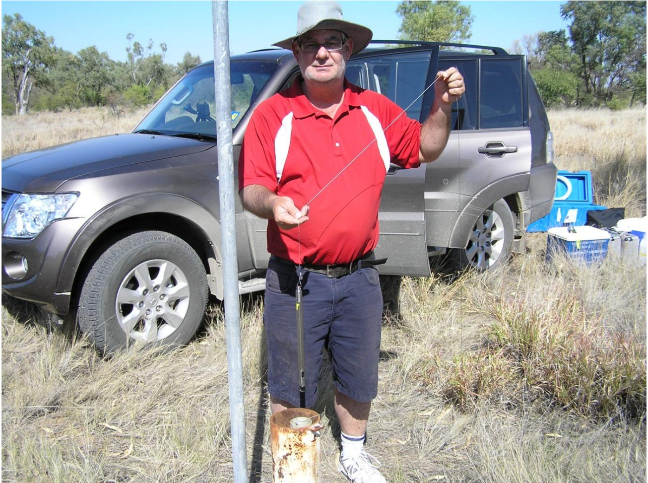
Figure 2.4 Installing a water level/salinity logger in an alluvial bore near Maxwellton during a field trip in August/September 2012
