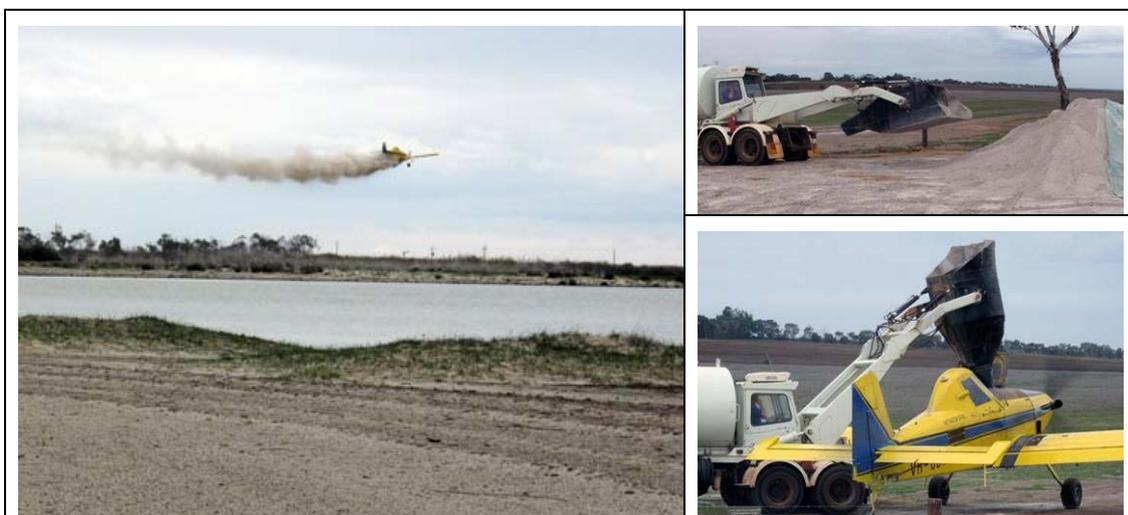
**Figure 6-2.** Aerial application of limestone in Boggy Lake, SA (left hand side photo) and photos on right land side showing mechanism used to upload fine agricultural limestone into the aircraft in a nearby paddock.
