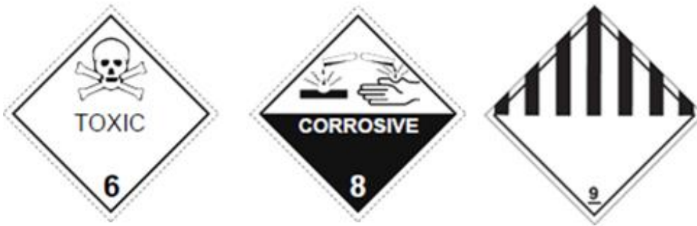
Figure 5: Example safety and hazard identifications labels and signage. Class 6: Toxic substances, Class 8 Corrosive substances, Class 9 Miscellaneous dangerous substances and articles [19]
