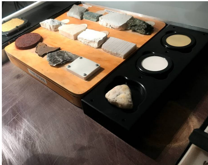
Figure 4 Test rocks plate with the wavelength standard plate alongside being scanned by a HyLogger3. A quartz pebble has been placed in the 3 rd slot in this example because this particular test rocks board lacks a quartz-rich sample.
