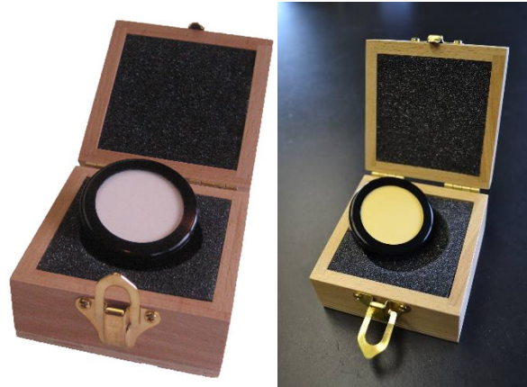
Figure 1 Manufactured wavelength standards (VNIR -left, MIR-TIR -right) from Middleton Research.
