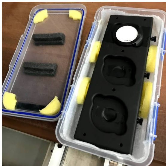
Figure 5 The wavelength standard holder in its case. In this example there is only a VNIR-SWIR wavelength standard (for a HyLogger1, which lacks a TIR sensor and, therefore, does not need the polystyrene on gold wavelength standard).
