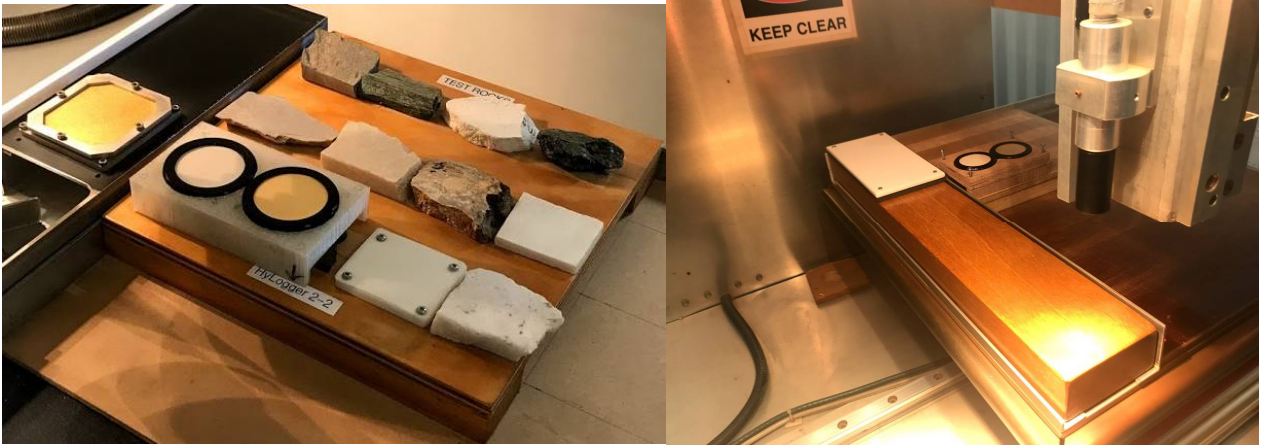
Figure 2 Example of the ‘concept wavelength standard holder’ mounted on a test rocks board, covering the iron oxide samples(left). The wooden wavelength standard holder being tested on a spare test rocks board (without rocks) before being placed on an operational test rocks board (right) on HyChips 6-2.
