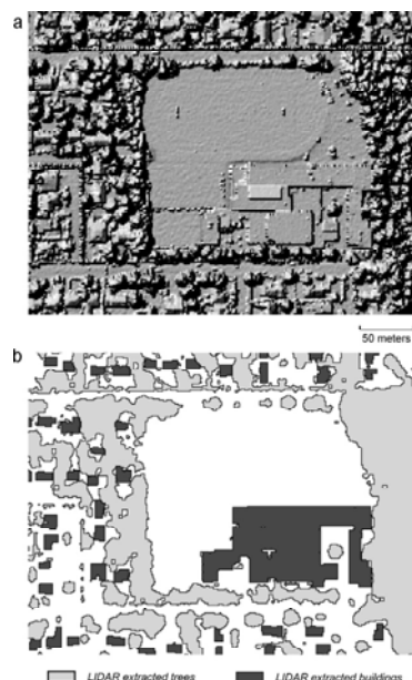
Figure 4-8. Maps depicting (a) a hillshade model of gridded LiDAR data and (b) the planar extent of trees and buildings form the LiDAR data
