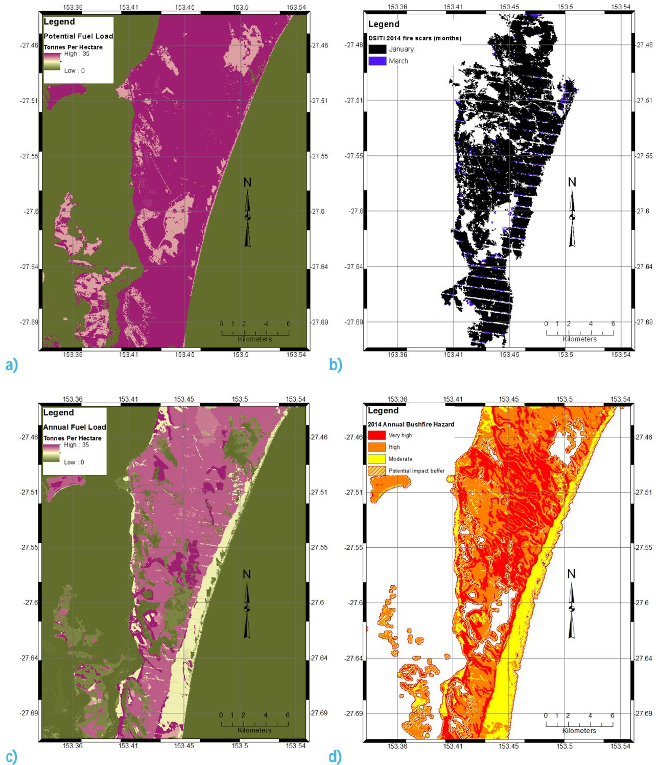
Figure 7: Demonstration of fire scar dataset artefacts and the impact on annual fuel load outputs a) potential fuel load, b) 2014 fire scar, c) 2014 annual fuel load and d) 2014 annual bushfire hazard.
