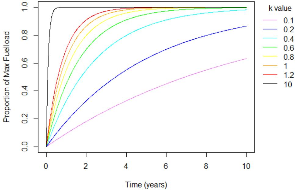
Figure 3: Examples of fuel accumulation towards steady state for different decomposition constant ( $k$ ) values.
