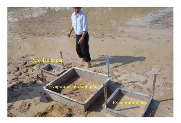
Figure 4: Installation of the percolation, evapotranspiration and evaporation pan.
