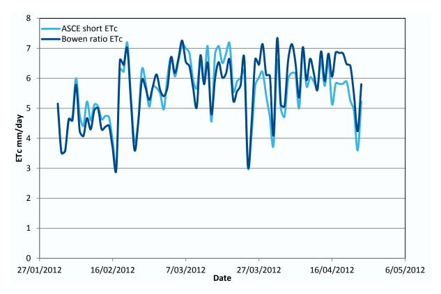
Figure 9: Daily crop evapotranspiration (ET<sub>c</sub>) using Bowen ratio and ASCE short approach for the period 1-Feb to 24 April 2012.
