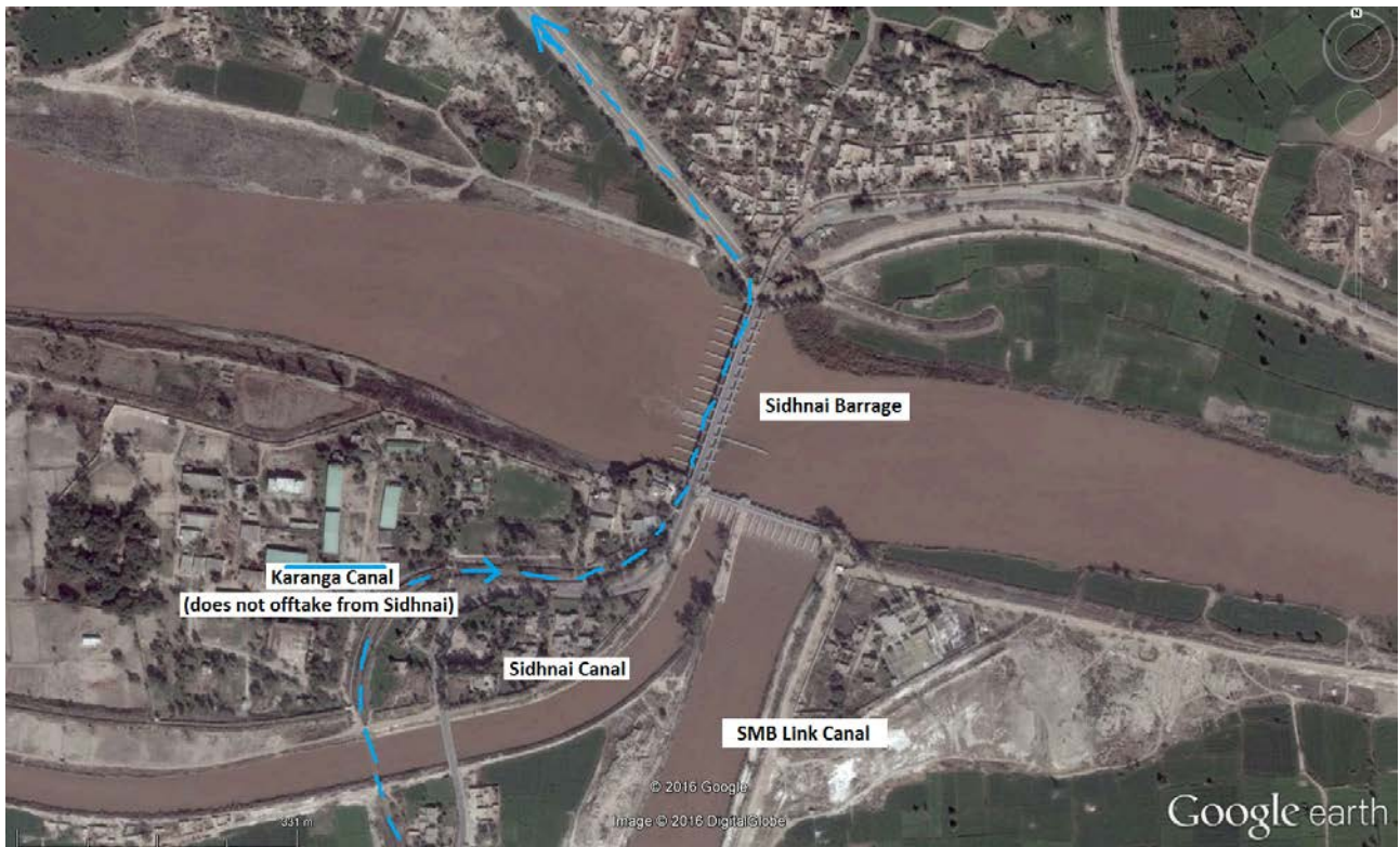
Figure 43 Sidhnai Barrage showing main barrage and offtake canals
