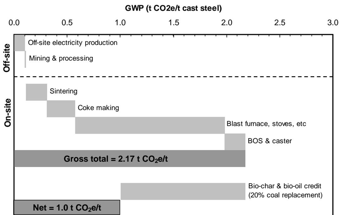
**Figure 4. GWP footprint of the integrated steel route (sintering) showing reduction from 20% replacement of coal with charcoal.**
