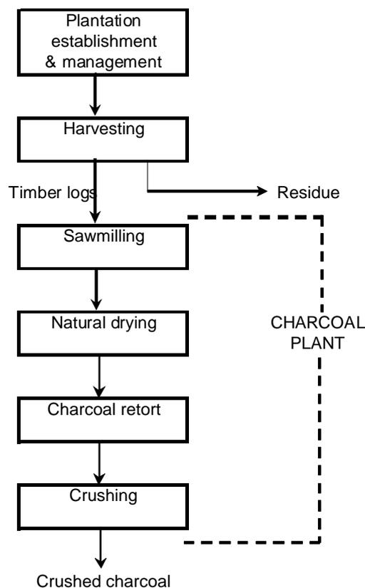
Figure 1. Schematic flowsheet of charcoal production.
