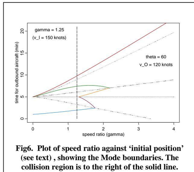
**Fig6. Plot of speed ratio against ‘initial position’ (see text) , showing the Mode boundaries. The collision region is to the right of the solid line.**
