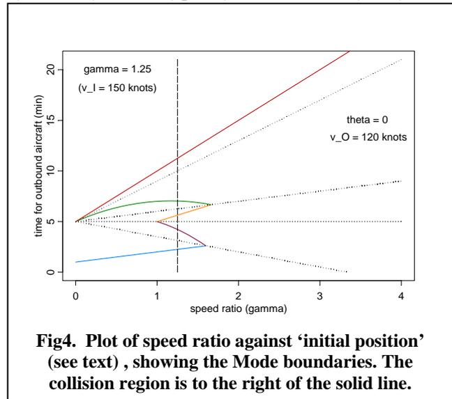
**Fig4. Plot of speed ratio against ‘initial position’ (see text) , showing the Mode boundaries. The collision region is to the right of the solid line.**
