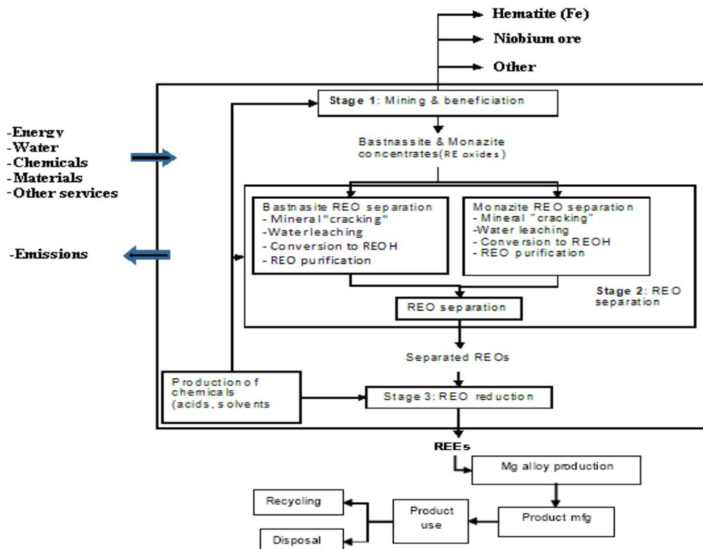
**Fig. 1. The "cradle-to-gate" LCA boundary for the production of RE metals**
