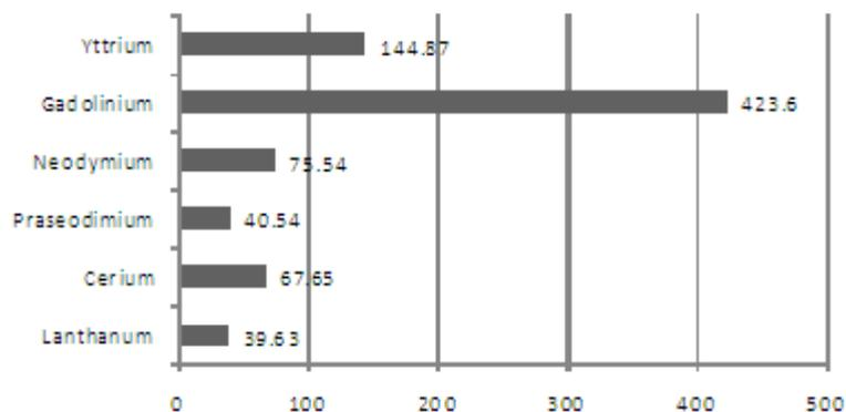
Fig.2. GHG emissions of RE elements (kg of CO<sub>2</sub> eq./kg of REE)
