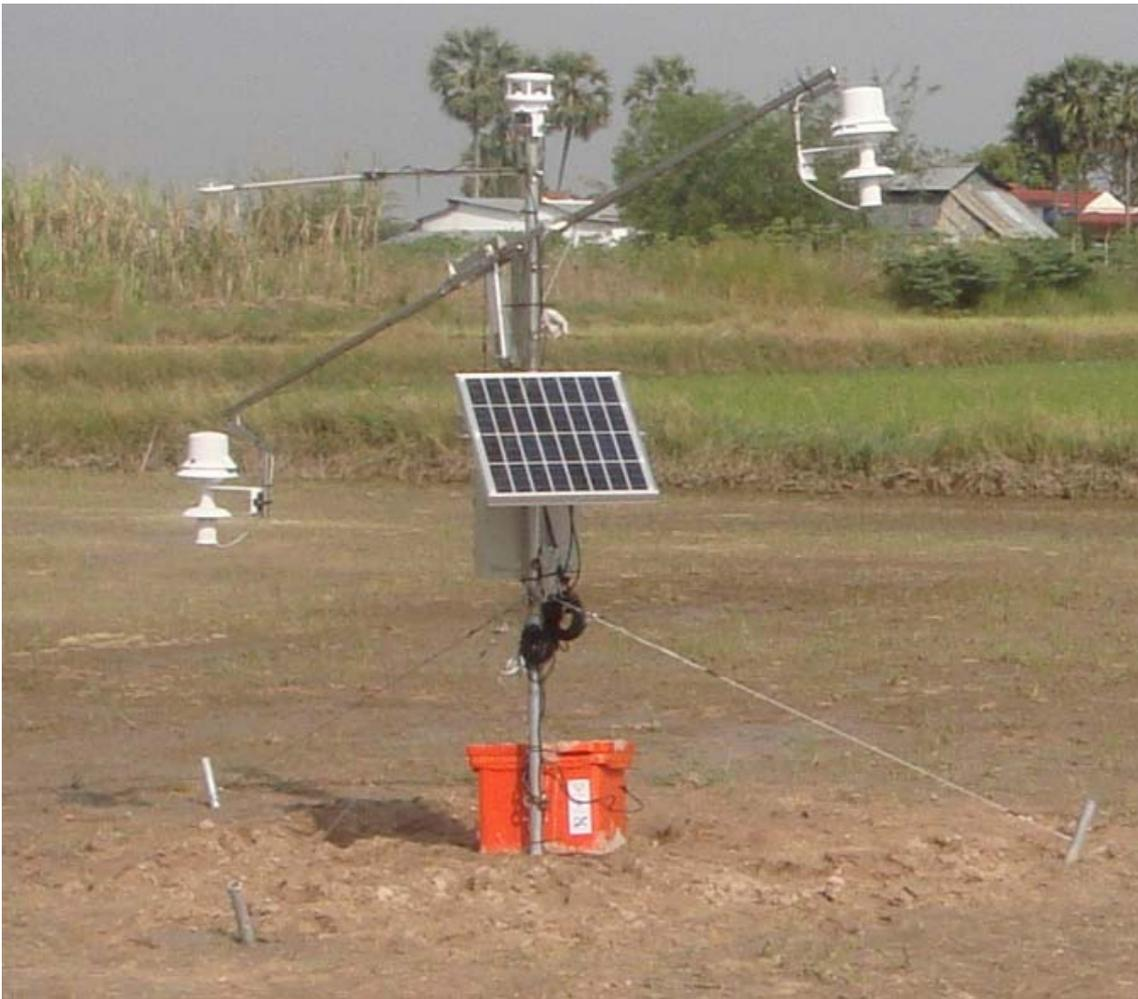
Figure 3: Installation of the Bowen ratio instrumentation on the 23<sup>rd</sup> January 2012.
