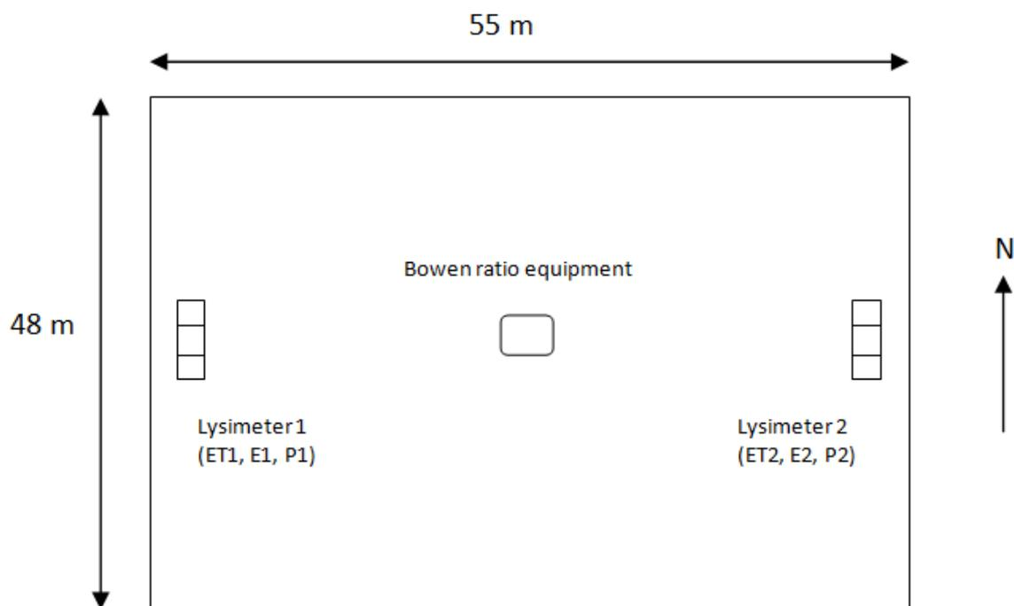
Figure 2: Experimental layout at CARDI field
