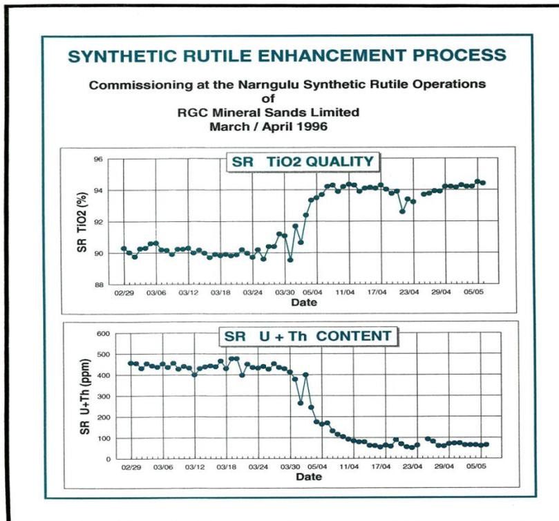
Figure 3. Plant log of the SREP process startup
