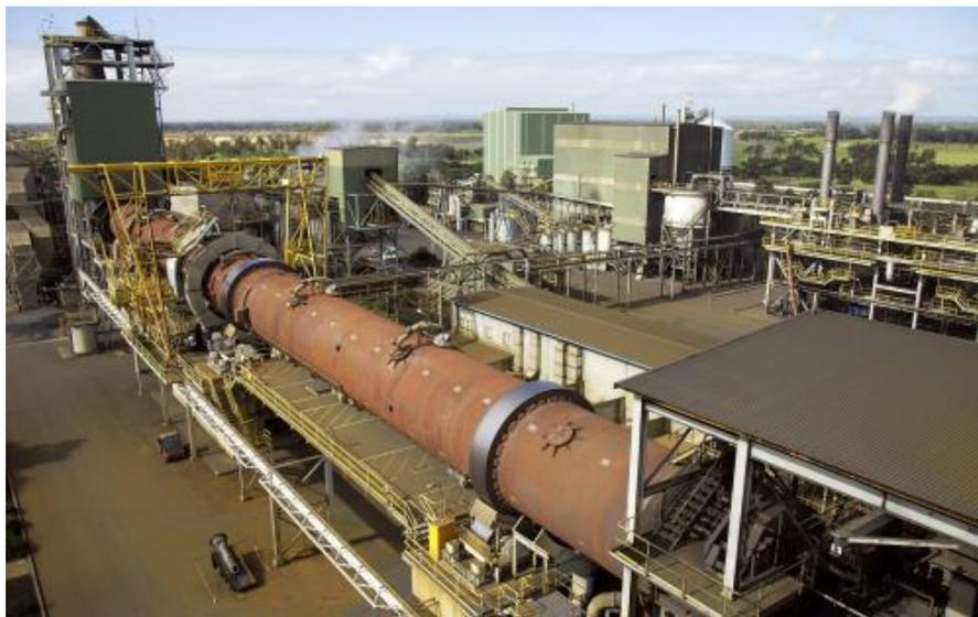
**Figure 1.** Commercial Becher reduction kiln.
